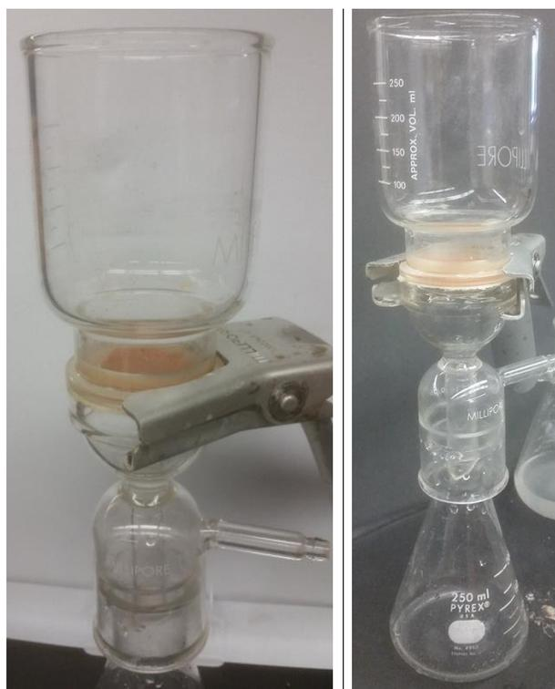
**Figure 14.** Figure showing filtration set-up for powdered samples supported on filter paper-supported sintered glass
