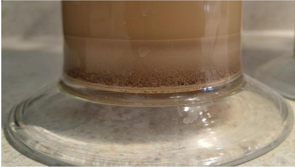
Figure 5-7. Detail photo of sediments settling at base of graduated cylinder. Note the fining upward sequence that develops as coarse particles fall out of suspension.
