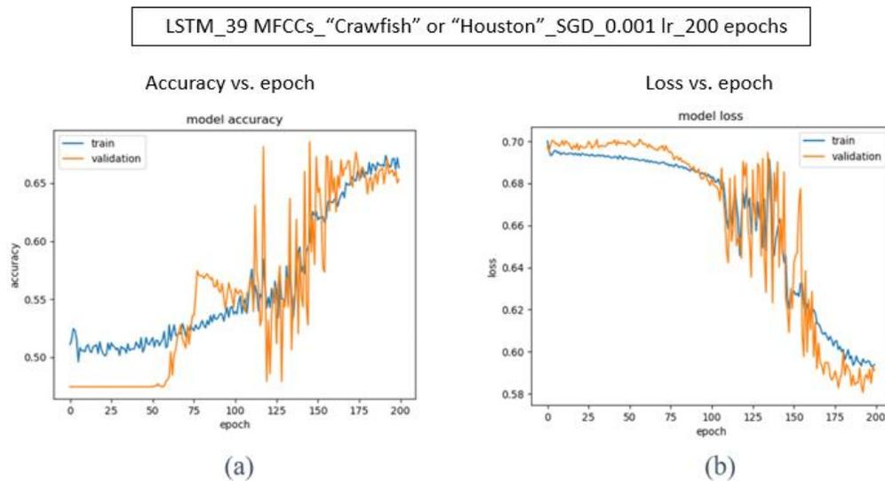
Figure 20: (a) Accuracy and (b) Loss Plots of the LSTM for 39 MFCCs with the SGD Optimizer, 0.001 for the Learning Rate, and 200 Epochs
