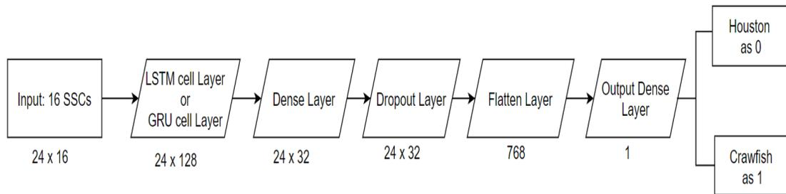
Figure 30: LSTM and GRU Model Structure for the “Houston” or “Crawfish” Classification Experiment with 16 SSCs
