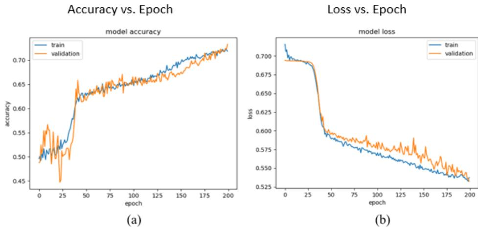
Figure 24: (a)Accuracy and (b) Loss Plots of the GRU for 39 MFCCs with the ADAM Optimizer, 0.001 for the Learning Rate, And 200 Epochs
