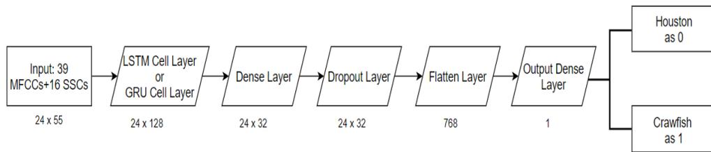
Figure 35: LSTM and GRU Model Structure for the “Houston” or “Crawfish” Classification Experiment with Combined 39 MFCCs and 16 SSCs
