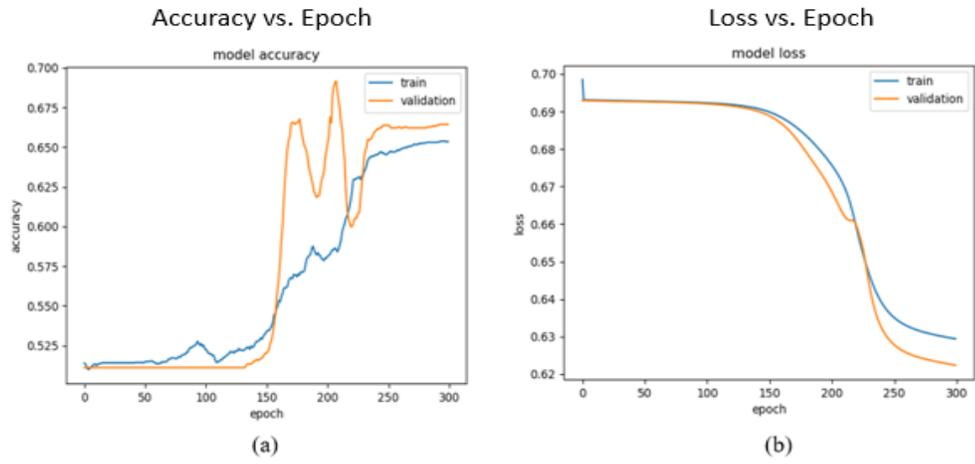
Figure 31: (a) Accuracy And (a) Loss Plots of The LSTM with 16 SSCs for ADAM Optimizer, 0.0001 for the Learning Rate, and 300 Epochs
