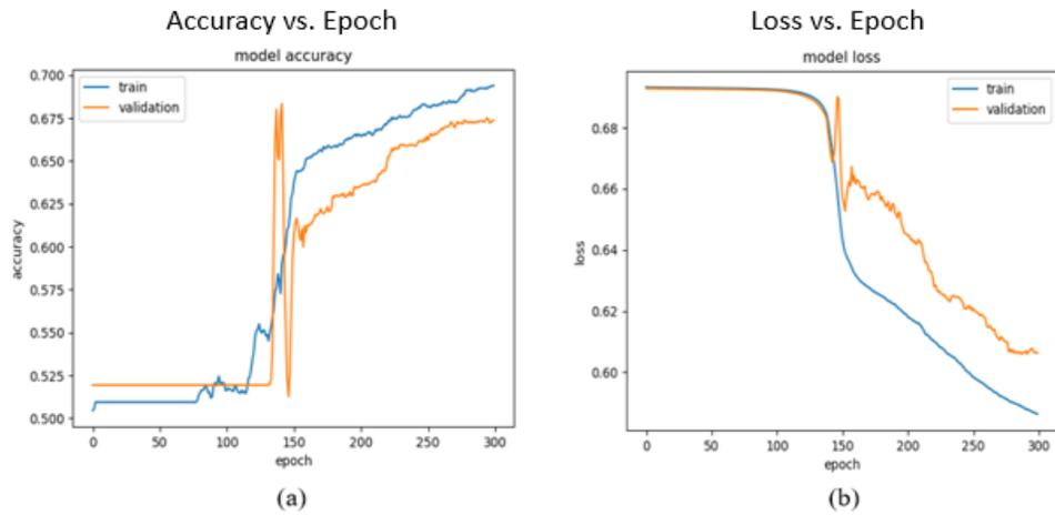
Figure 32: (a) Accuracy and (b) Loss Plots of the GRU with 16 SSCs for the ADAM Optimizer, 0.0001 for the Learning Rate, and 300 Epochs
