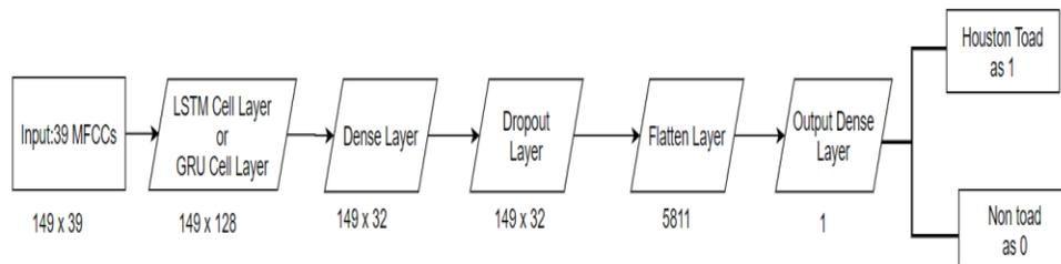
Figure 12: The LSTM and GRU Model Structure for the “Houston toad” or “Non-toad” Classification Experiment with 39 MFCCs
