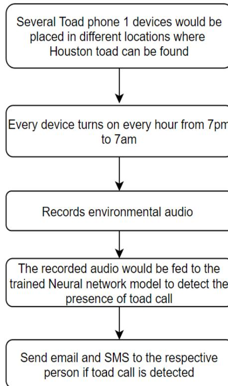
Figure 2: Flowchart Demonstrating the Working Principle of the Toadphone 1
