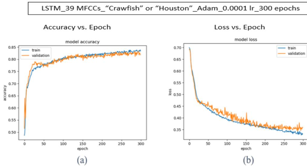
Figure 26: (a) Accuracy and (b) Loss Plots of the LSTM and 39 MFCCs with the ADAM Optimizer, 0.0001 Learning Rate, 300 Epochs
