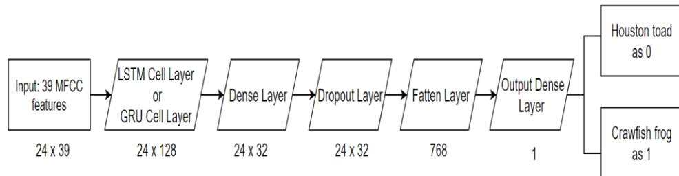
Figure 19: LSTM and GRU Model Structure for the “Houston” or “Crawfish” Classification Experiment with 39 MFCCs
