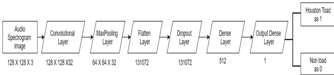
Figure 17: CNN Model Structure for the “Houston toad” or “Non-toad” Classification Experiment with Mel-Spectrogram Images
