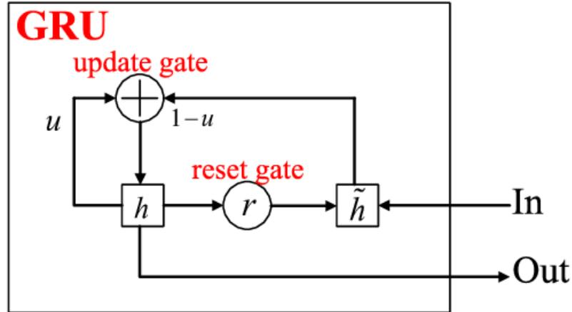
Fig. 7: GRU Internal Architecture [22]
