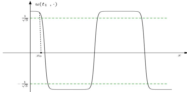
FIGURE 7. Solution  $u$  for  $t = t_1$ . The solution now belongs to the hyperbolic zone, i.e.,  $p'(u(t_1, x)) > 0$  for almost every  $x \in \mathbb{R}$ . We recall that  $p(u) = (u^2 - 1)u$ .
