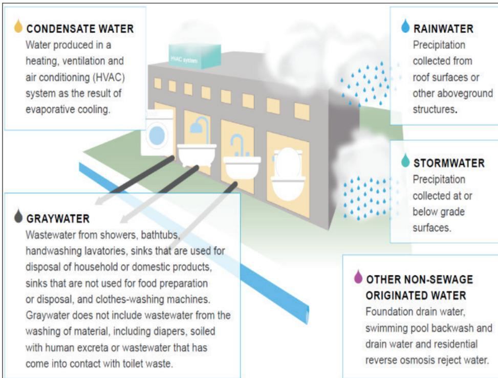
**Figure 5.** Different sources of water in an urban setting (Source: Austin Water)
