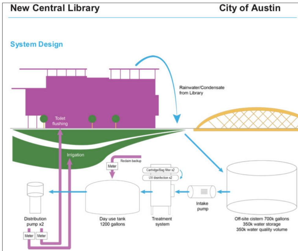
**Figure 6.** Rainwater and AC condensate collection and treatment system at the City of Austin’s Central Library (Source: Austin Water, Alternative Water Systems)
