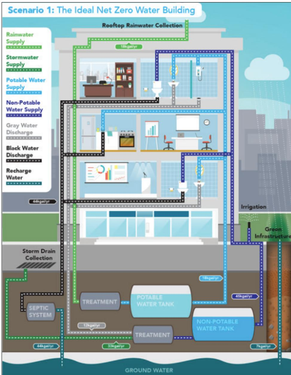
**Figure 4.** The ideal net zero water building (Source: U.S. Office of Energy Efficiency and Renewable Energy)
