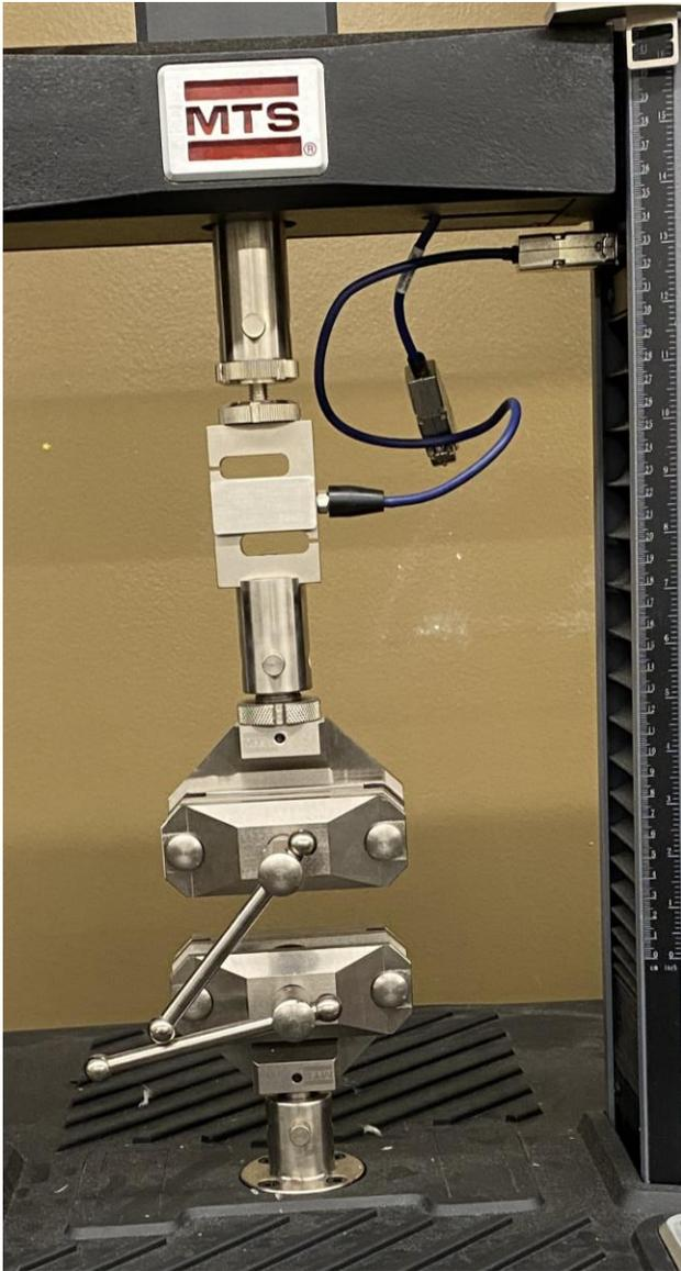
Figure 45: Mechanical tensile testing equipment used for thin films deposited on PET substrate
