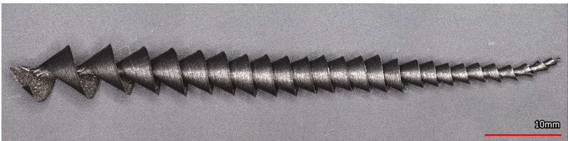
Figure 3.15: Long continuous chip from drilling as-cast 65-45-12 ductile iron.
