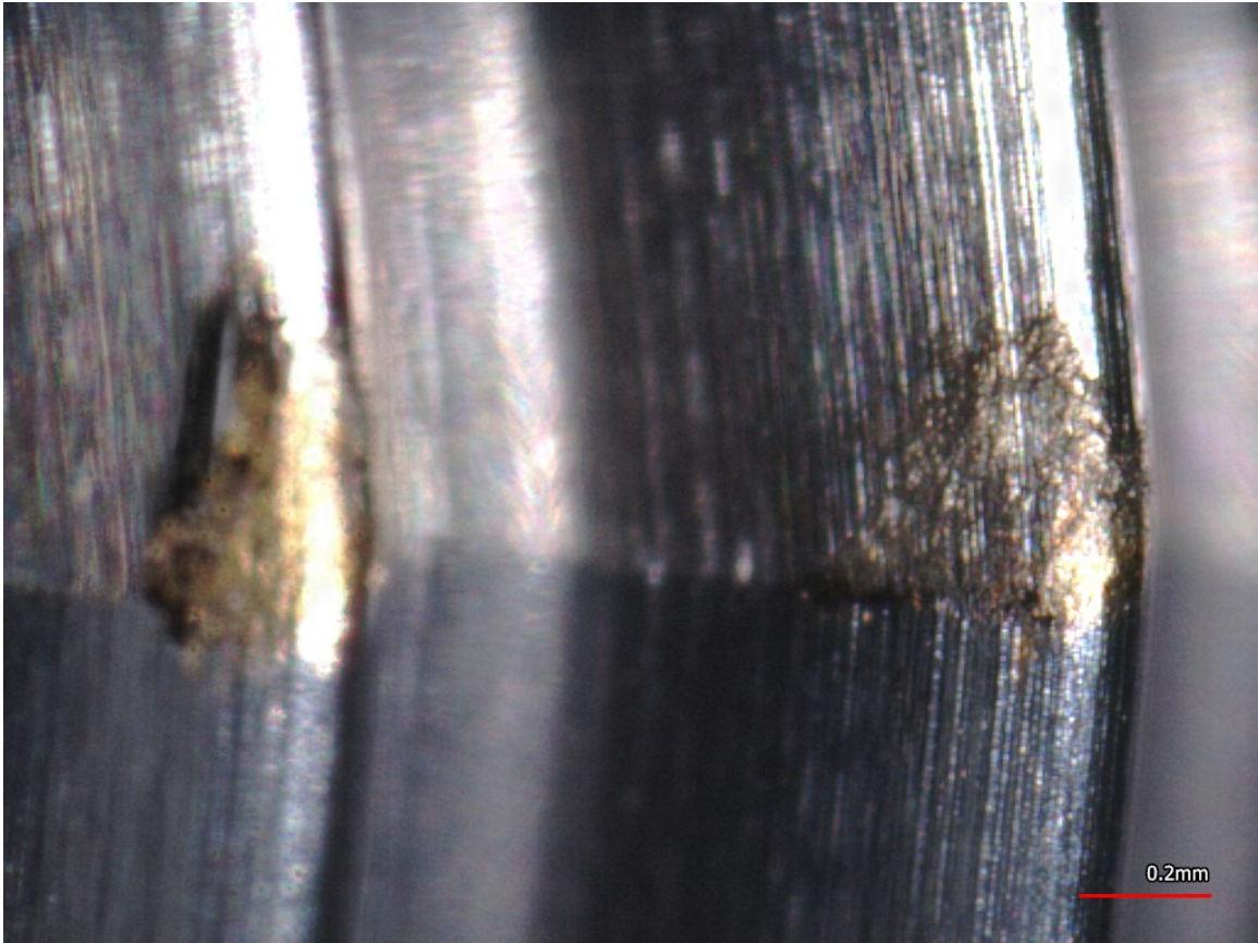
Figure 3.6: Form tap lobe wear after 28 holes. Appears to show less wear than the flutes of the cut tap.
