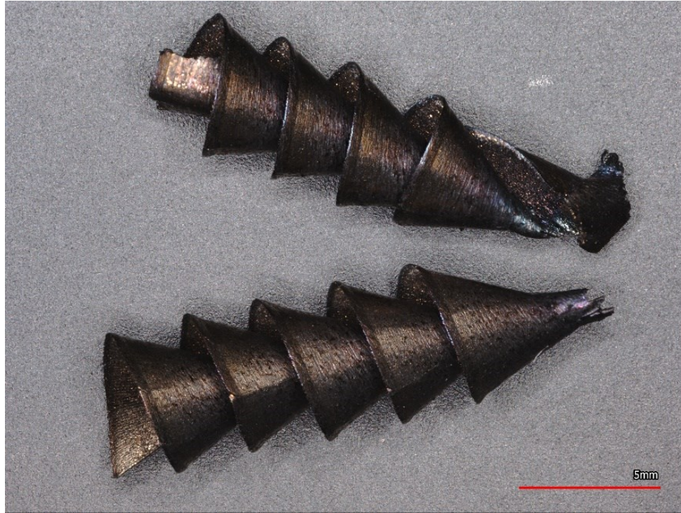
Figure 3.13: Medium length continuous ADI chip from drilling. Note the serrations at the point.
