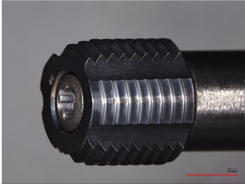
Figure 3.4: Lobe wear on the form tap insert after 28 holes.
