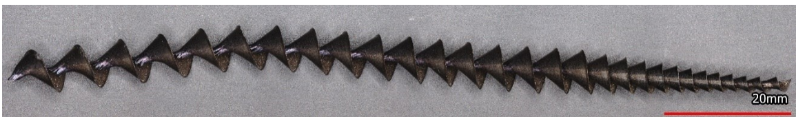
Figure 3.14: Long continuous ADI drilling chip curling along a constantly tightening spiral.
