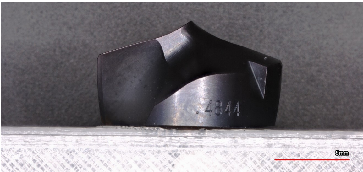
Figure 3.7: An unused carbide drill insert. Cutting rake face on the left side.
