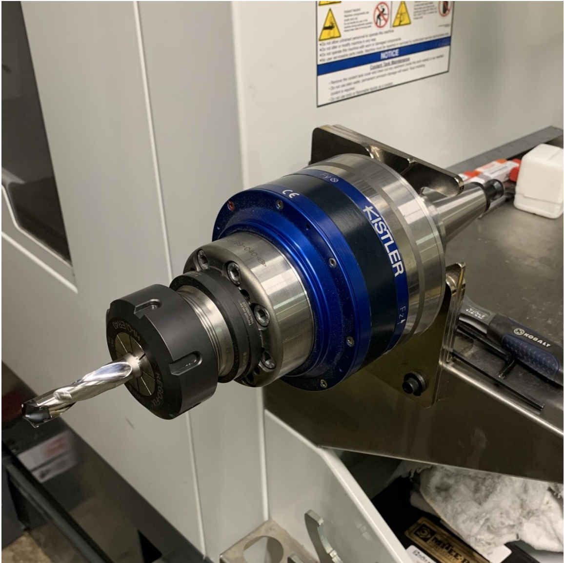
Figure 2.4: Kistler Type 9170-A rotating dynamometer with carbide insert drill.
