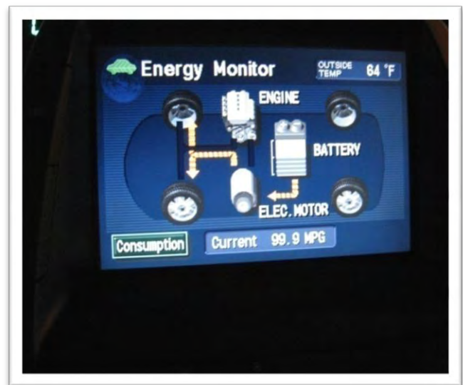
Image 2.7: This is the drivers panel that shows when the vehicle is operating on the combustable engine, the electric motor or operating on battery power alone.
