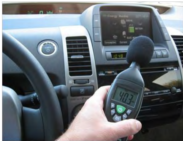
Image 4.4: Decibel meter reads 40.3 inside the hybrid at idle, a very low reading for a passenger vehicle.
