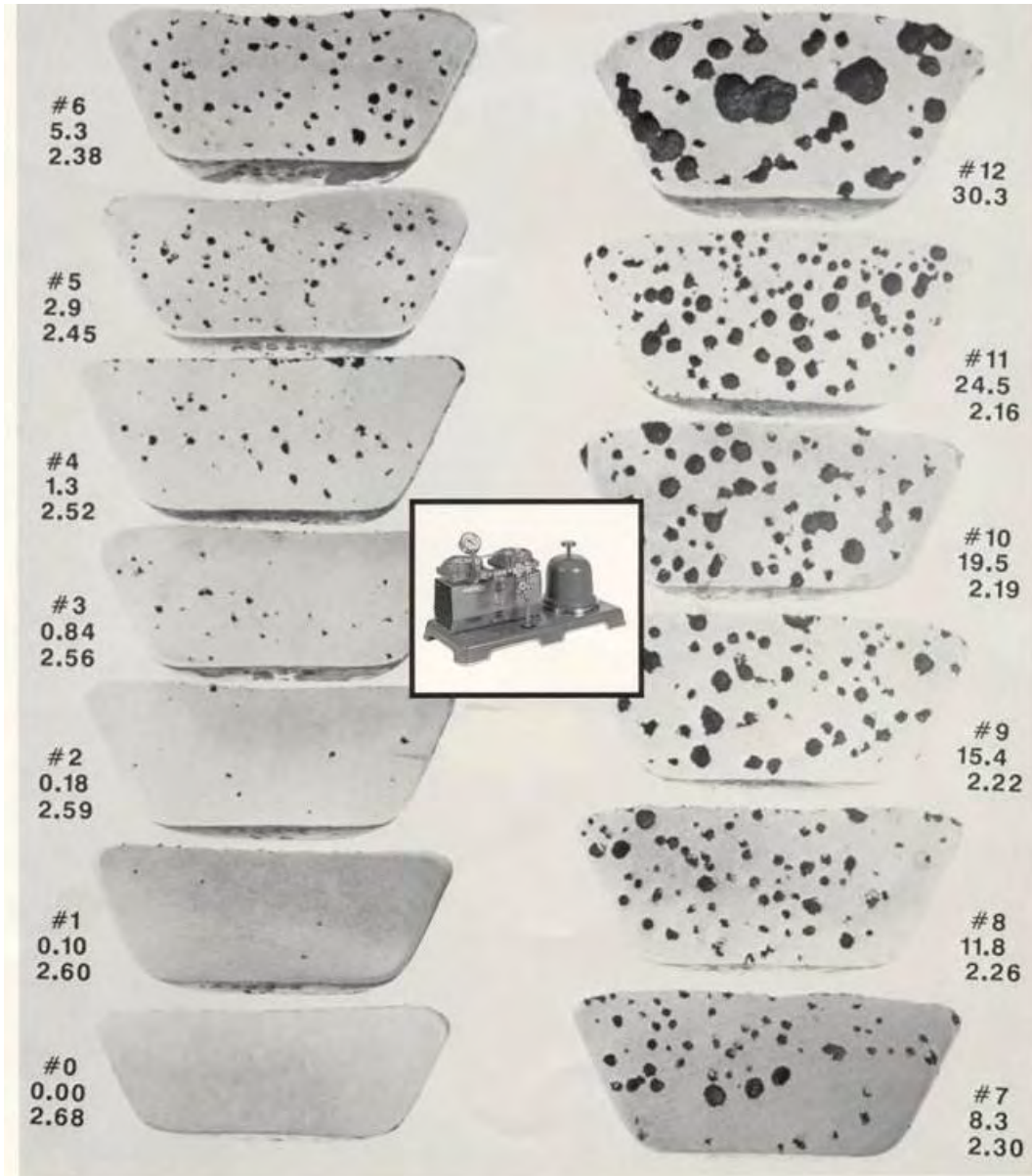
Figure 8. Aluminum Comparative Standards for Gas (100 mm pressure).
