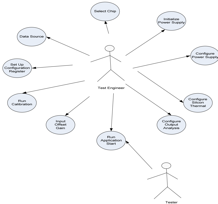
Figure 70 Test Engineers and Testers Relationship to Automatic Test Environment
