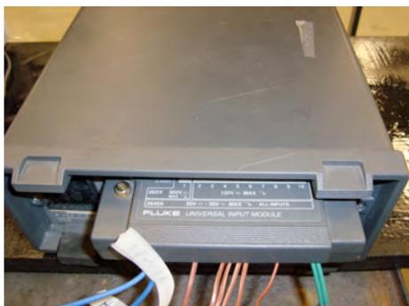
**Figure 3.2.7: Cartridge inserted in back of Hydra**
