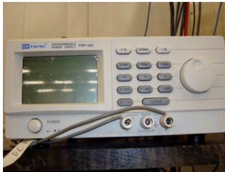
**Figure 3.2.2: Instek Programmable Power Supply**
