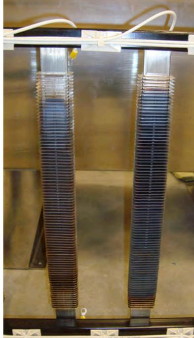
**Figure 3.2.12: Finned heaters**
