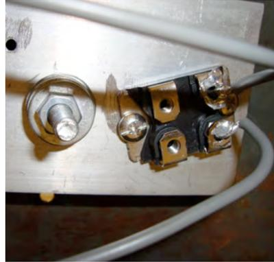
**Figure 3.2.5: Shunt resistor (0.01 Ohm)
