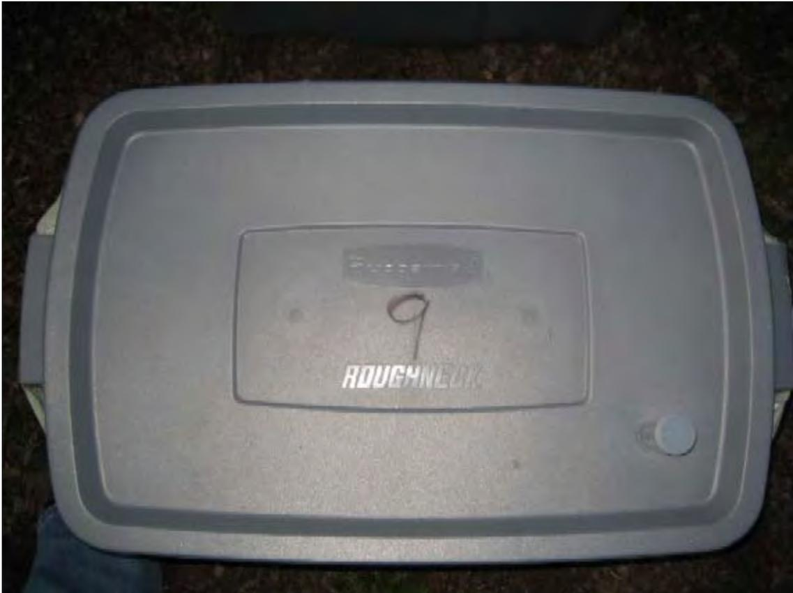
**Figure 1: Photograph of Container 9. This photograph is illustrating the number system on the lids and the airlock in the bottom right corner of the lid.**
