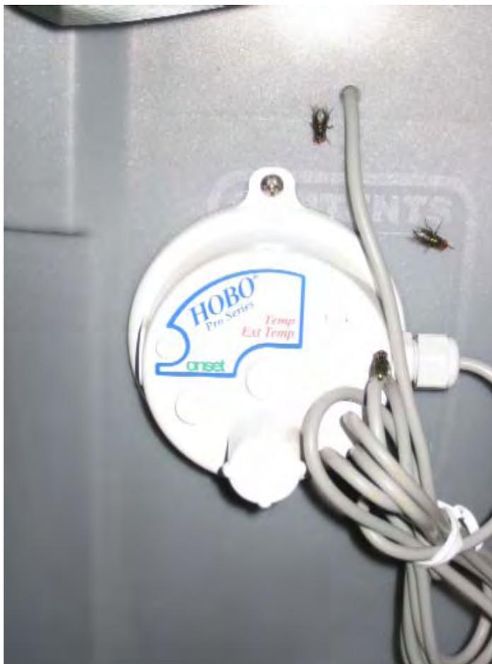
**Figure 2: Photograph of the HOBO® H8 Pro Temperature Logger. The Logger is attached to Container 9.**
