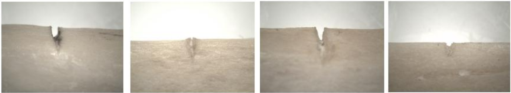
Figure 7: Examples of the kerf shapes seen in the experiment. Please see Appendix B for additional examples.
