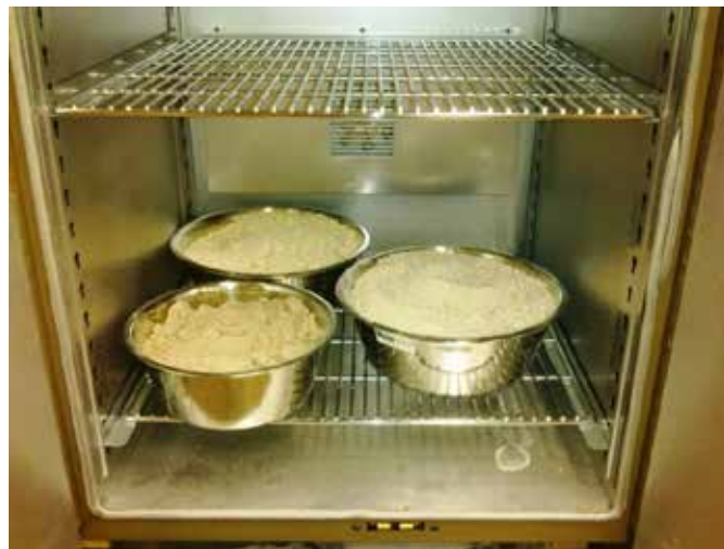
Figure 3-6. Fine aggregates in the oven
