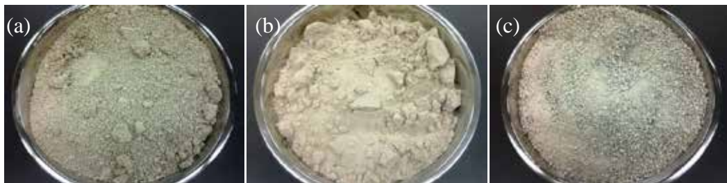
Figure 3-1. Fine aggregates. (a). manufactured sand; (b). silica sand; and (c). FRCA
