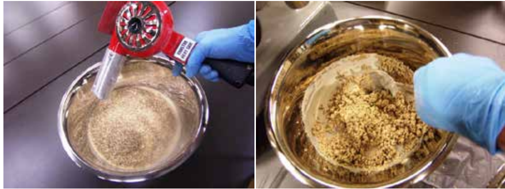
Figure 3-4. Drying and stirring fine aggregates sample
