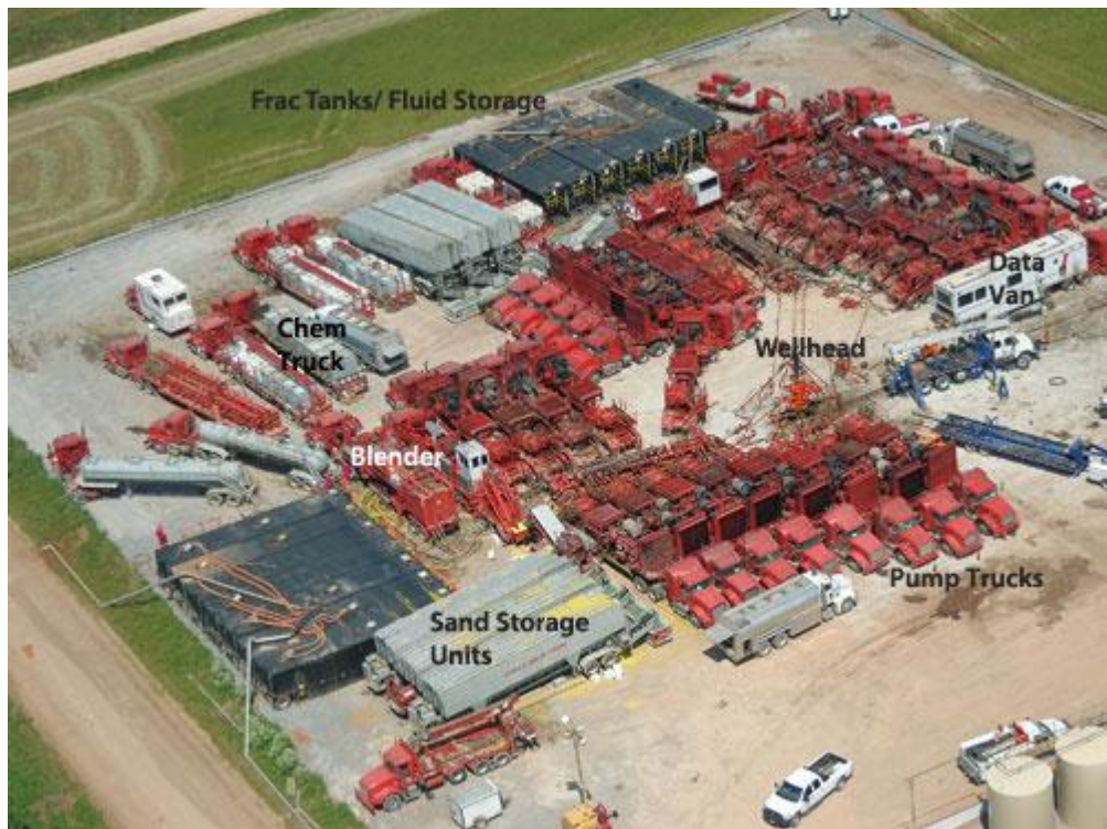
Figure 1. Typical site set up (Frac Focus 2012).
