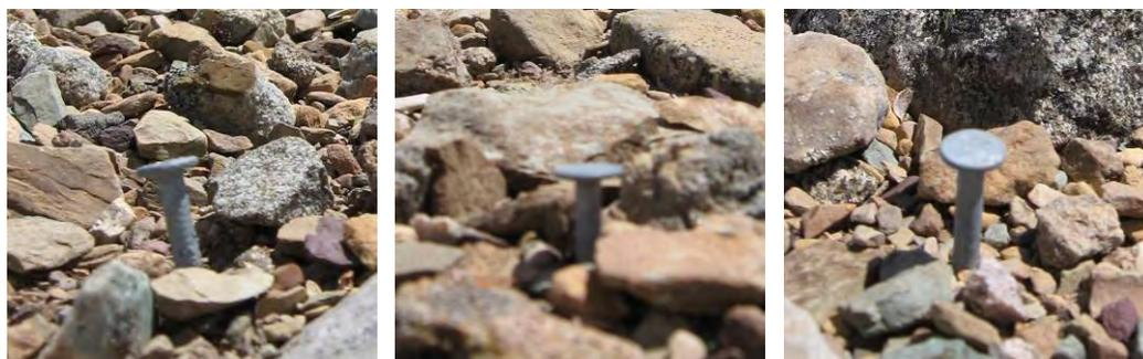
**Figure 84. Examples of heaved nails, Site I, SP, 2006.**
