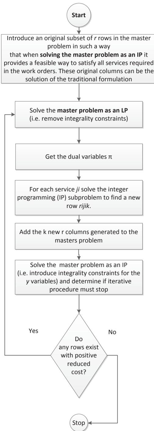
Figure 1. Flowchart of the column generation process.
