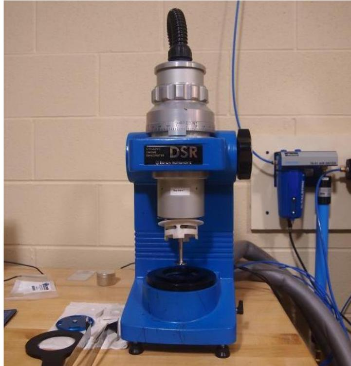
Figure 8. Dynamic Shear Rheometer (DSR)
