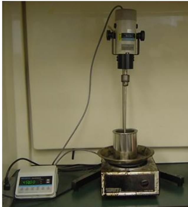
Figure 4. CRM binder blending setup
