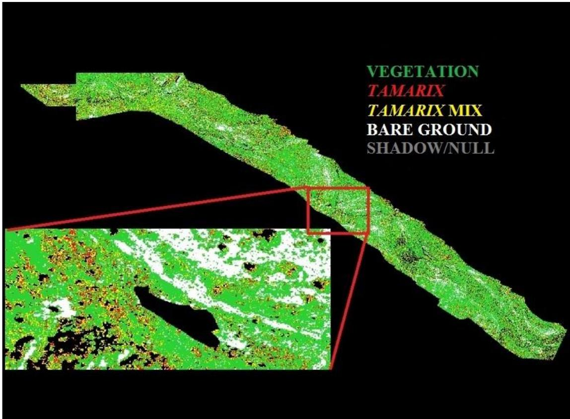
Figure 11. Final classification output from UAV-derived true color imagery.
