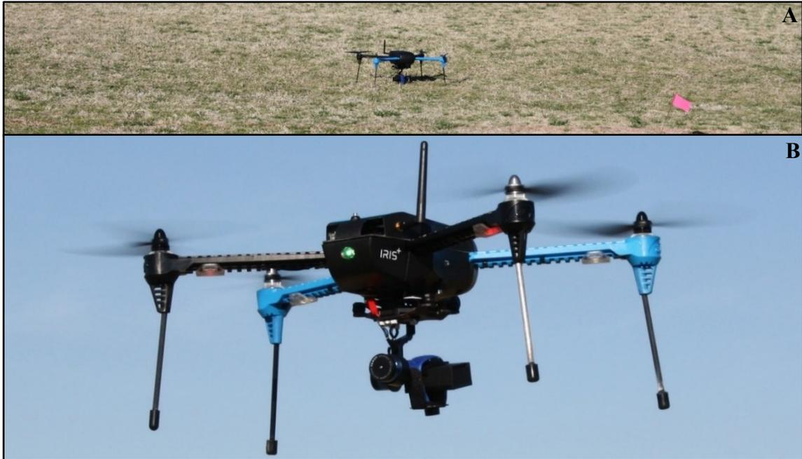
**Figure 3.** 3DR IRIS+ quadcopter sUAS. (A) 3DR IRIS+ prior to takeoff in a test area. (B) 3DR IRIS+ in flight with 3-axis gimbal on bottom mounted with GoPro4 Black camera/3.6mm low distortion lens.
