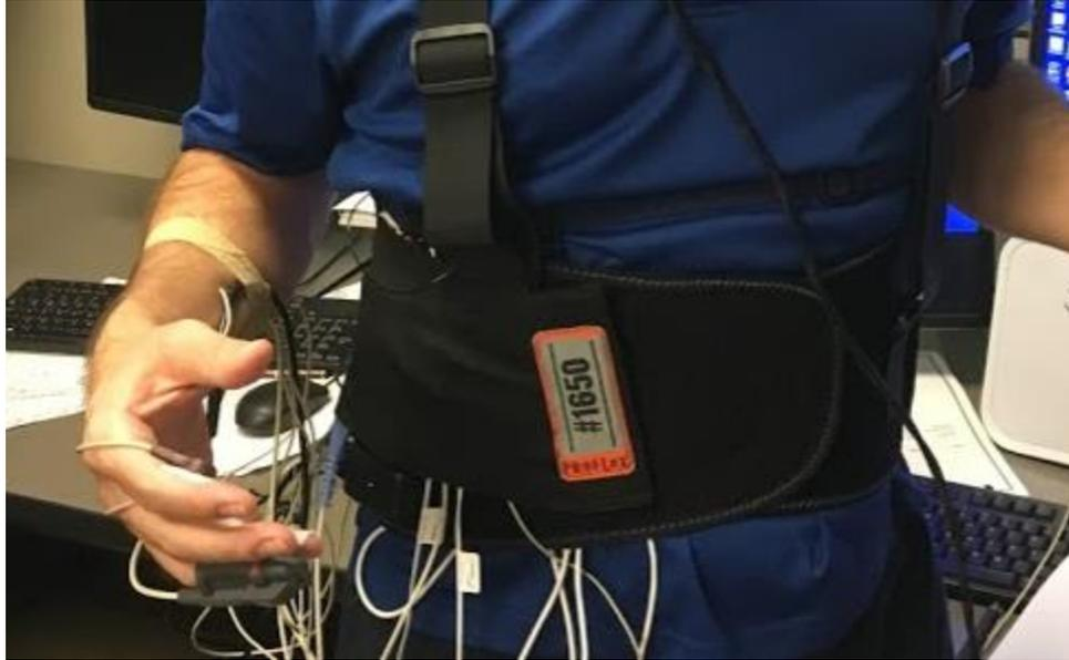
Figure 4: Body BioRadio mounting with Back Support Belt
