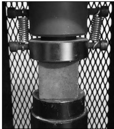
**Figure 4.5 Setup for Compressing Mortar.**
