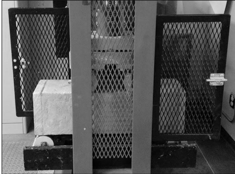
**Figure 5.11 Setup for Flexing Concrete.**
