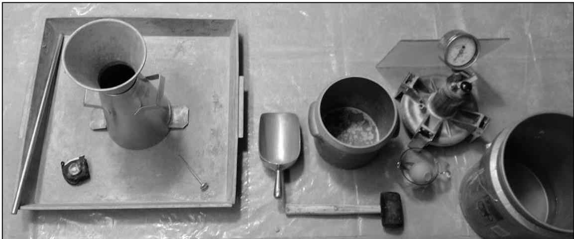
**Figure 5.2 Slump Cone, Thermometer, Air Meter and Associated Tools.**
