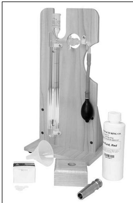
**Figure 2.1 Blaine Air Permeability Apparatus.**
