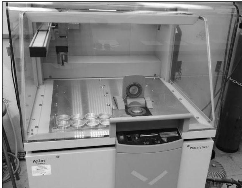
**Figure 2.9 Panalytical Axios X-Ray Fluorescence Spectrometer.**
