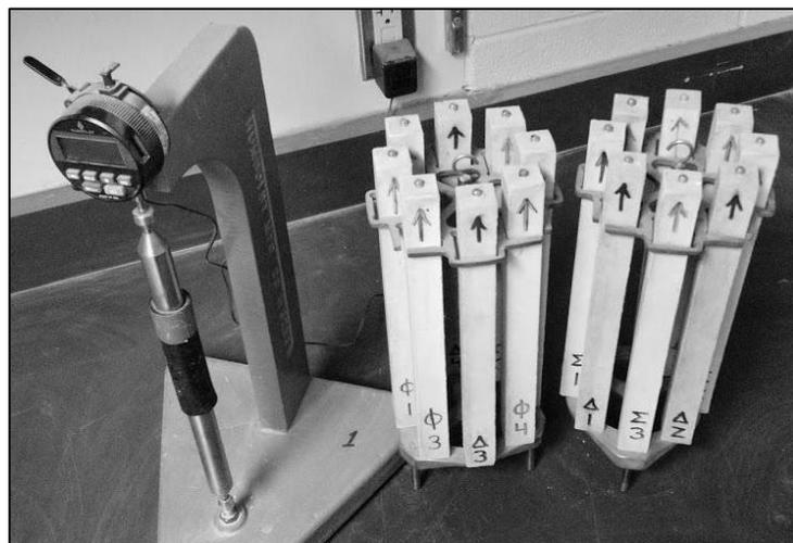
**Figure 4.7 Length Comparator and Mortar Prisms.**
