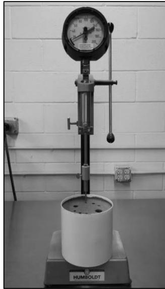
**Figure 4.3 Acme Mortar Penetrometer.**
