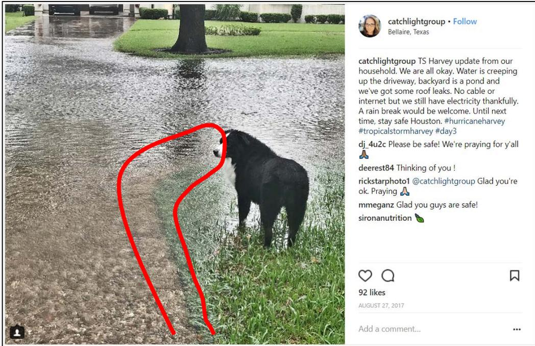
**Figure 4. An Example of Extracting Water Level from a Picture Using the Surrounding Physical Objects. The Red Line Shows the Edge Between the Road and the Sidewalk.**
