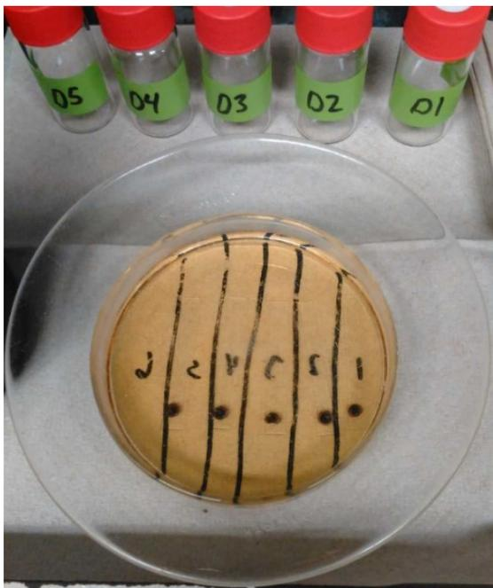
Figure 51: Image of poly(ProDOT-Bu<sub>2</sub>) films submerged in ethanolamine
