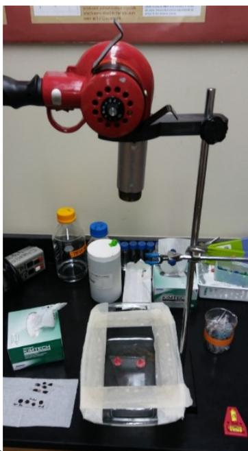
Figure 24: Experimental setup to enhance film drying rate. Heat gun has hot and cold settings as well as two airflow settings (High and Low)
