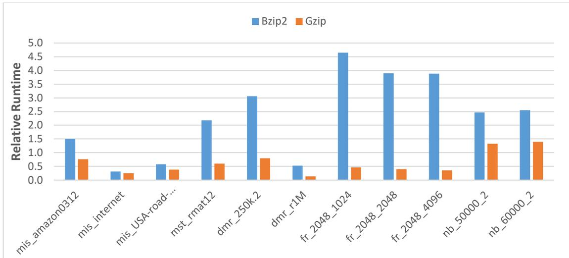
Figure 10. Runtime of Bzip2 and Gzip relative to runtime of ECL-Tracer
