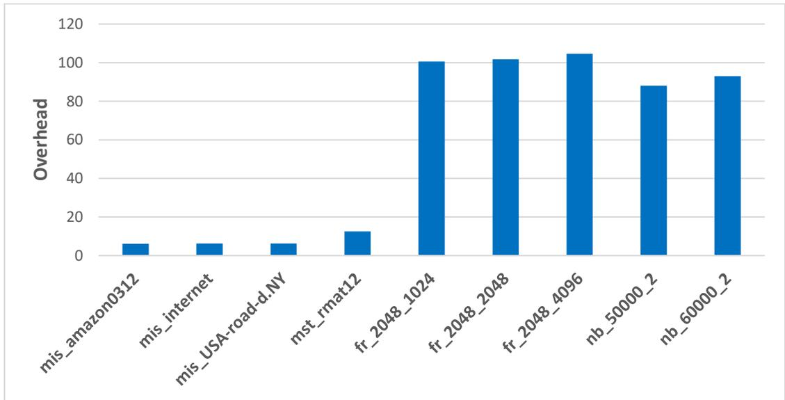
Figure 11. ECL-Tracer overhead relative to using no tracing tool on K40
