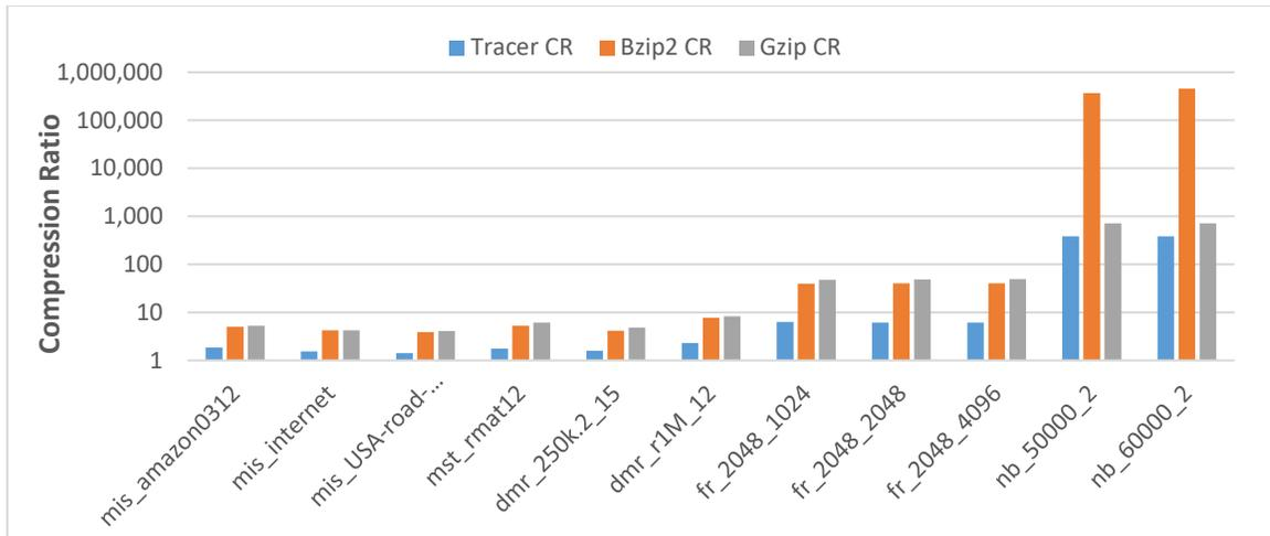
Figure 9. Compression ratios for ECL-Tracer compared to Bzip2 and Gzip
