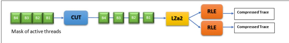
Figure 2. Diagram showing the application of CUT in the chain of compression components
