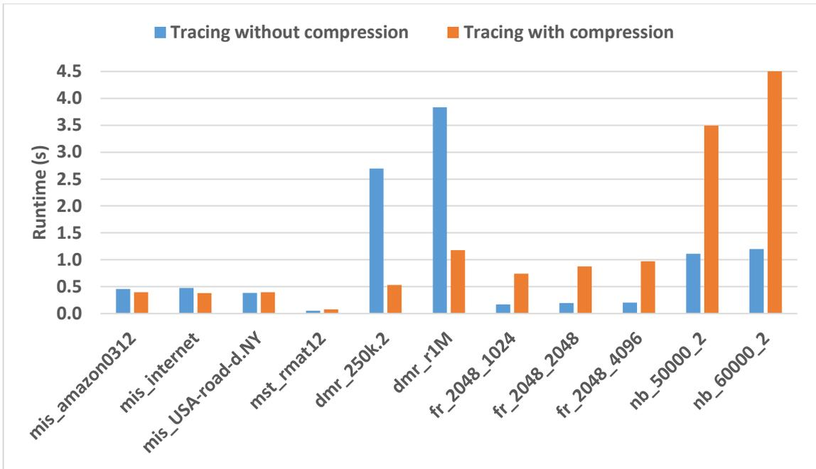
Figure 6. Runtimes of ECL-Tracer with and without compression
