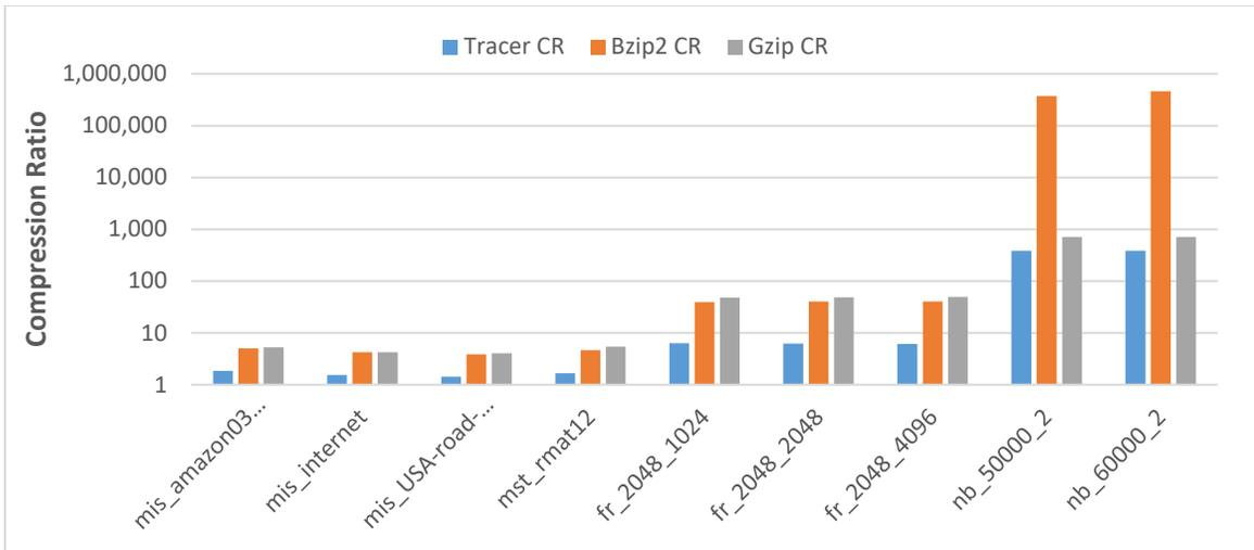
Figure 15. Compression ratios for ECL-Tracer compared to Bzip2 and Gzip on K40
