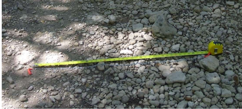
Figure 4. Demonstration of chain-length method of measuring roughness. Note the chain in front of the tape measure with orange tape at the ends.
