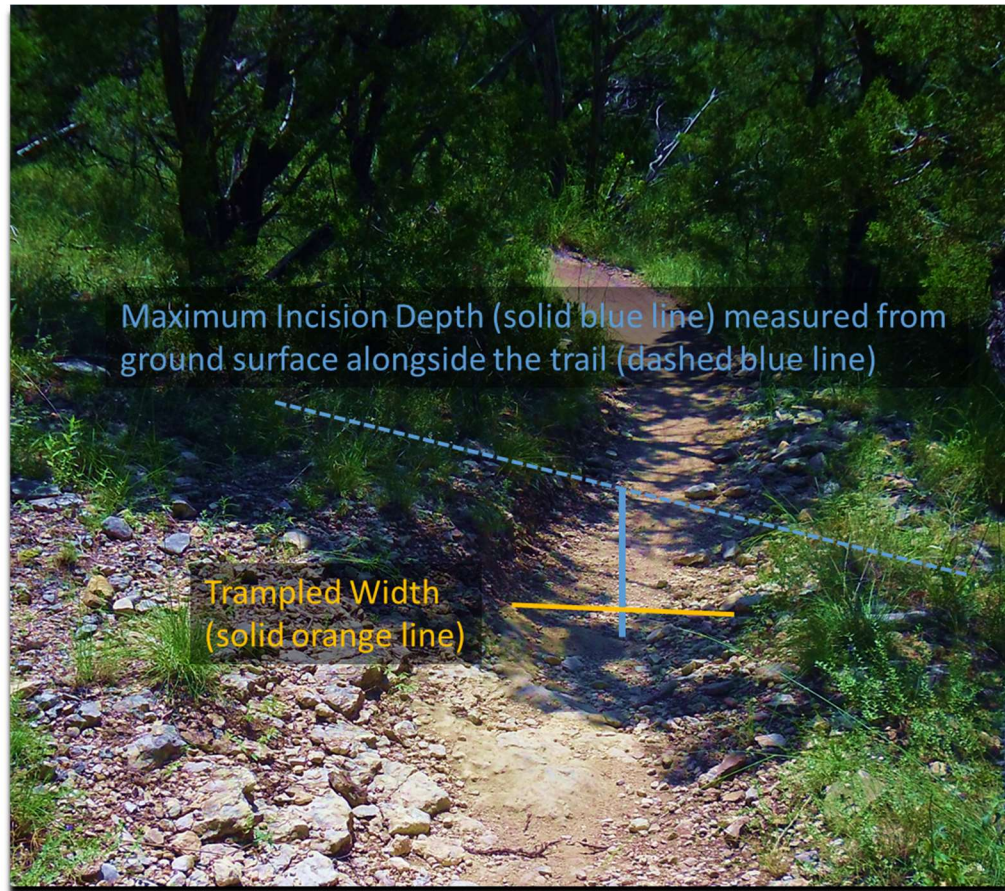
Figure 3. Depiction of trampled width and maximum incision depth measurements.
