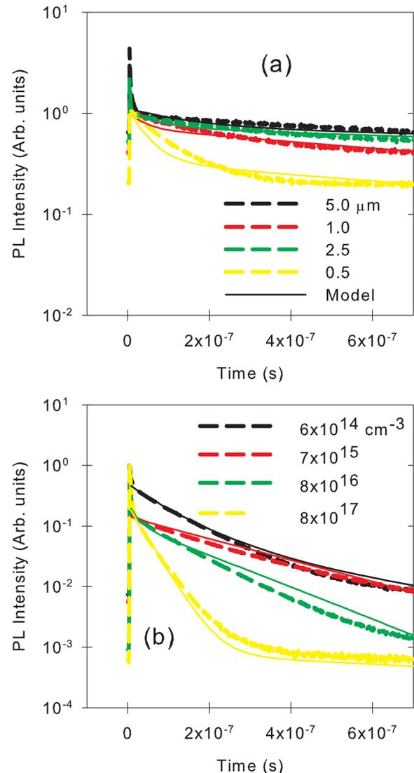
FIG. 1. TRPL traces shown for (a) undoped double heterostructures of several different thicknesses and (b) 1  $\mu\text{m}$  thick samples of several different iodine doping concentrations. Each solid line represents a modeled time dependence.
