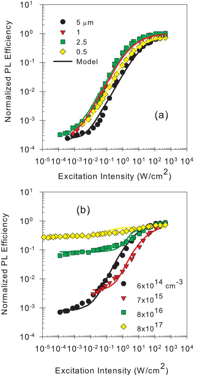
FIG. 3. Ratio of PL intensity to laser excitation incident at the sample surface ( $I$ ), plotted as a function of the excitation, for (a) undoped double heterostructures of several different thicknesses and (b) 1  $\mu$ m thick samples of several different iodine doping concentrations. Each solid line represents a modeled intensity dependence.
