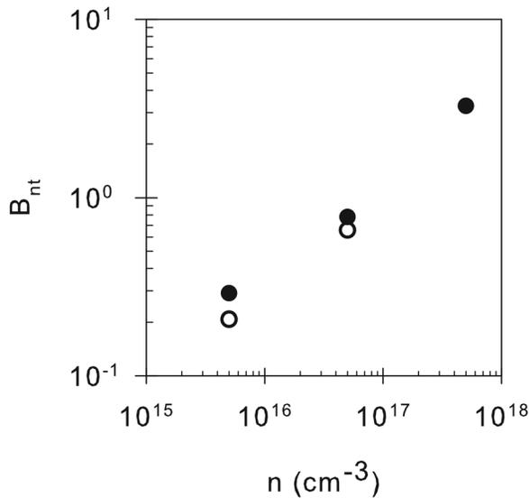
FIG. 4. The quantities  $B_{nt}$ , calculated from the maximum slopes in Fig. 3, are plotted vs. carrier concentration in DHs with 1  $\mu\text{m}$  (filled) and 2  $\mu\text{m}$  (empty) CdTeSe absorber layers.
