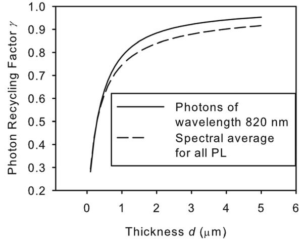
FIG. 2. The photon recycling factor for CdTe absorber layer as a function of thickness. The factor is also shown with the approximation of monochromatic PL emission at 820 nm.
