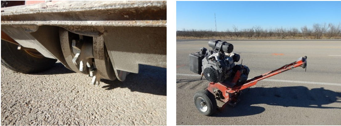
Figure 2-4. Carbide-tipped rotary impact router bit
