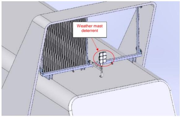
**Appendix, Figure 1.** Image depicting the position of the deterrent array on the weather mast facing off the rear of the nacelle at Los Vientos during deterrent testing in 2017. Orientation shows the unit pointed towards the leeward side of the nacelle. This unit was removed during deterrent testing in 2018.
