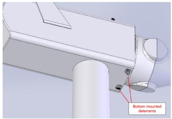
**Appendix, Figure 3.** Image depicting the position of deterrent arrays located on the bottom of the nacelle, upwind at Los Vientos during deterrent testing in 2017. Orientation shows units pointed towards leeward side of the nacelle.
