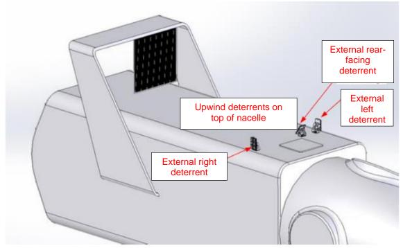
**Appendix, Figure 2.** Image depicting the position of deterrent arrays located on top of the nacelle, upwind at Los Vientos during deterrent testing in 2017. Orientation shows the external rear-facing deterrent pointed towards the leeward side of the nacelle.
