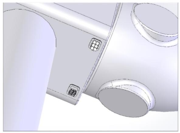
**Appendix, Figure 4.** Image depicting the new orientation of the bottom-facing deterrent arrays repositioned towards the rotor swept area at Los Vientos Wind Energy Facility during deterrent testing in 2018.
