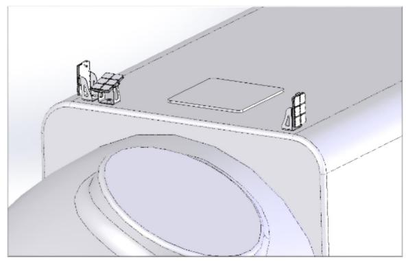
**Appendix, Figure 5**. Image depicting the new orientation of the top mounted deterrent arrays repositioned towards the rotor swept area at Los Vientos Wind Energy Facility during deterrent testing in 2018.
