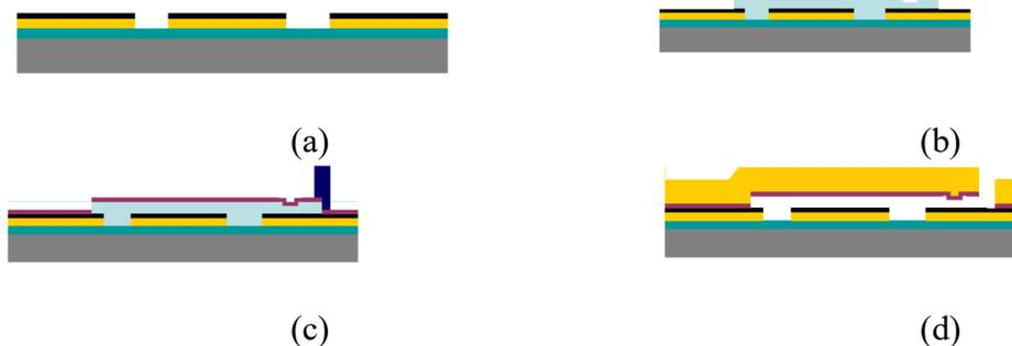
Figure 14. Switch process flow. (a) deposition and patterning of bottom electrode. (b) deposition and patterning of sacrificial layer. (c) deposition of top electrode as cantilever beam(d) plating cantilever beam, removing sacrificial layer to release the beam [48]
