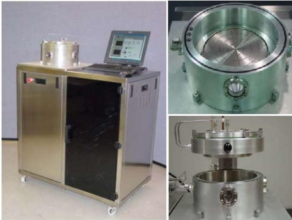
Figure 12. Typical RIE chamber for oxygen plasma treatment while plasma treatment [46]
