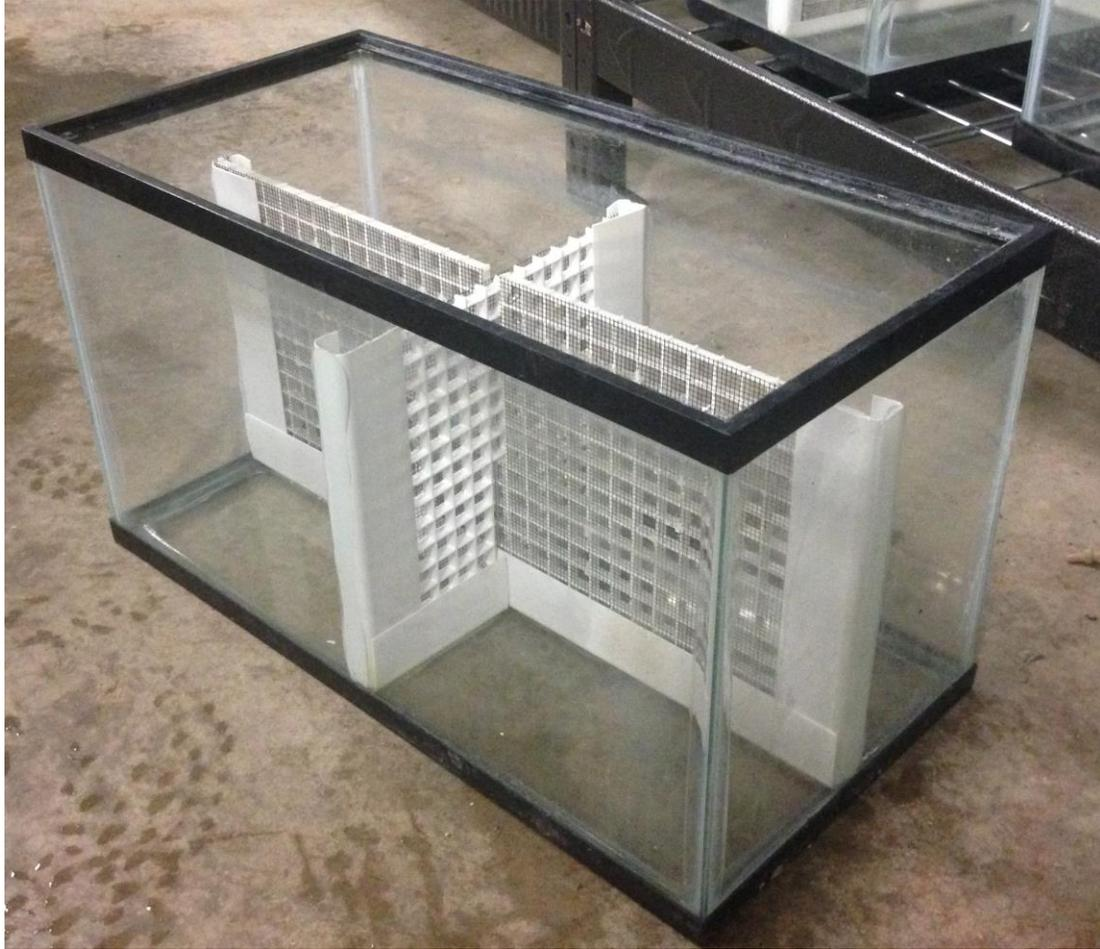
Figure 6. Experimental fish aquarium with partitions and U-channel installed.
