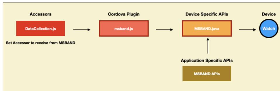
**Figure 15.** Fall detection App to Receive Sensor Data from MSBAND Smartwatch
