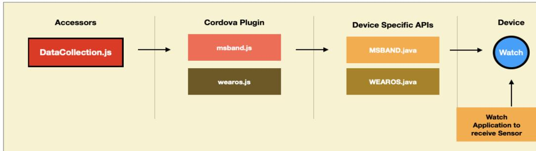
**Figure 11.** Data Collection Accessor Architecture
