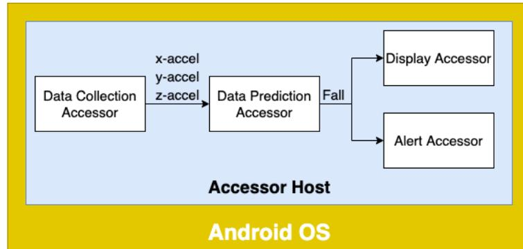
**Figure 8.** Main Accessors Used for the Fall Detection App
