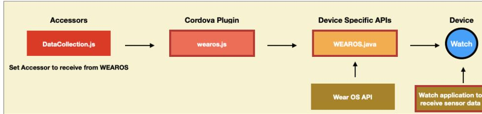
**Figure 16.** Fall detection App to Receive Sensor Data from WEAROS Smartwatch
