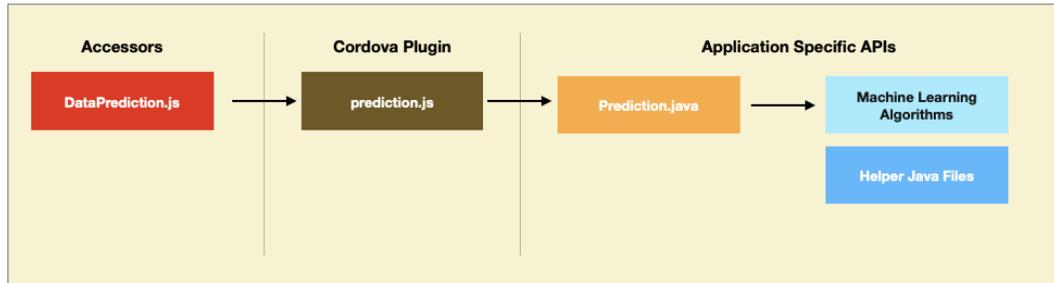
**Figure 12.** Data Prediction Accessor Architecture for the Fall Detection App
