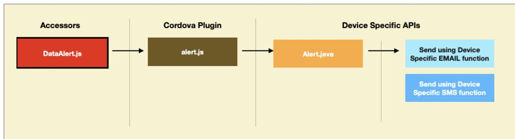
**Figure 14.** Alert Accessor Architecture
