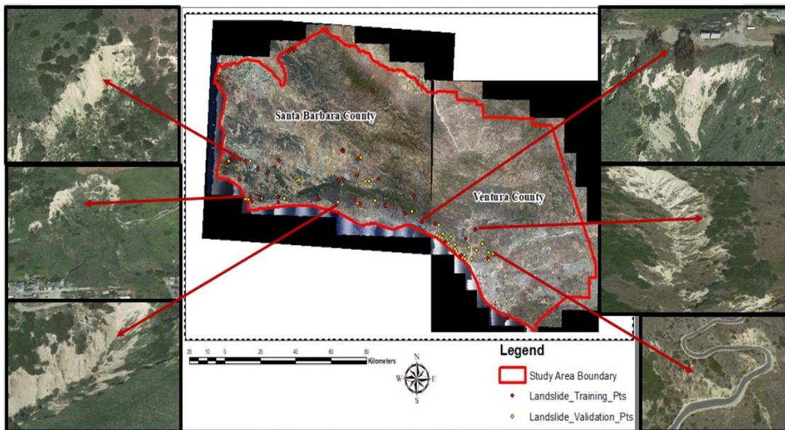
**Figure 10. Hill Shaded Map Indicating Landslide Locations and Landslide Examples Visually Interpreted and Identified on a High-Resolution Aerial Imagery.**
