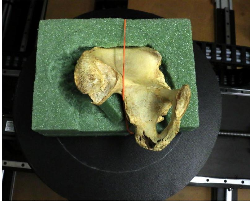
**Figure 0.5** - Specimen mounted for scanning placed on the scanning stage in the North Star scanner. View from above. X-ray source is to the left.
