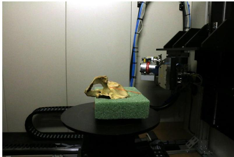
**Figure 0.4** - View of a specimen mounted for scanning from outside the North Star scanner. X-ray source is to the right.
