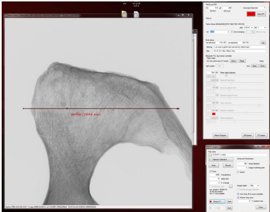
**Figure 0.6** - Technique development window from the NSI EFXDR software showing the radiograph of a specimen prior to scanning.
