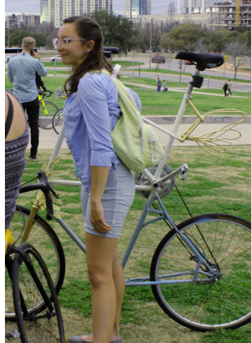
Figure 1 – A tall bike modification. Multiple frames welded on top of each other along with other corresponding modifications making the bike usable, otherwise known as a tall bike, is one fairly common example of a bicycle hack. This tall-bike and rider participated in the group ride event for the SXSW premier of Bikes vs. Cars (2015) in Austin, Texas. Photo Credit: Roger Lara Jr.
