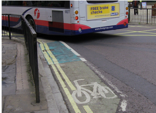
Figure 7 - A poorly designed bicycle lane. When cycling infrastructure is treated as afterthought the results are often full of fatal flaws, such as grating, curbs, debris, cars and car doors, bollards, and in some cases trees and other ridiculous obstacles. This clearly inadequate green lane was located in Central York, United Kingdom circa 2010. Photo Credit: Freewheeler, Crap Cycling and Walking in Waltham Forest , retrieved on June 16, 2016 ( http://crapwalthamforest.blogspot.com/2010/07/classically-bad-cycle-lane.html ).
