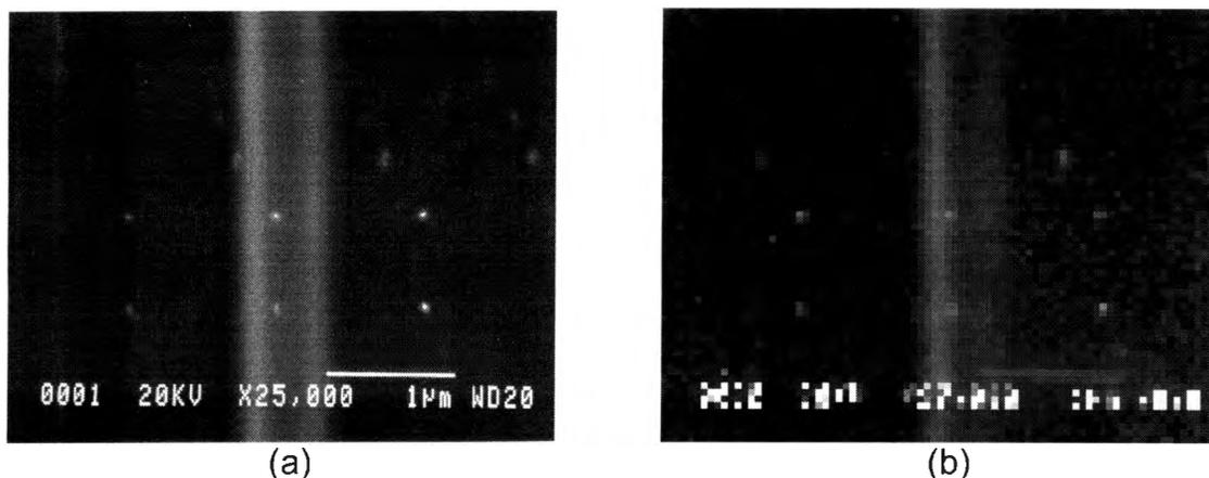
**Figure 4.7** SEM micrographs of: (a) **1** with 1% BPO and (b) **2** with 1% BPO exposed by using a 20 kV electron beam at an average beam current of 1.2 nA
