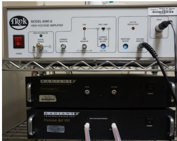
Figure 2.11: (b) Precision LC II ferroelectric test system from Radiant technologies inc.
