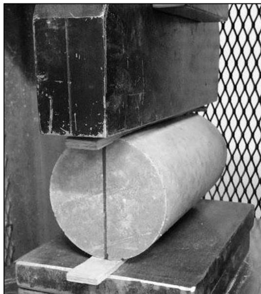
**Figure 5.9 Setup for Splitting Concrete.**
