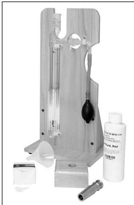
**Figure 2.1 Blaine Air Permeability Apparatus.**
