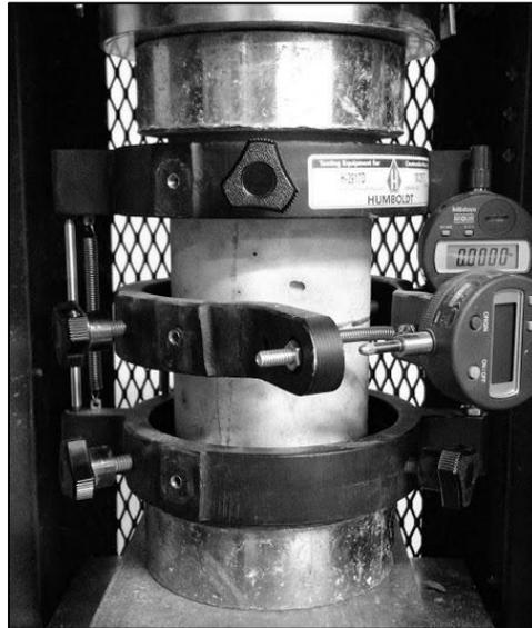
**Figure 5.14 Setup for Elastically Deforming Concrete.**
