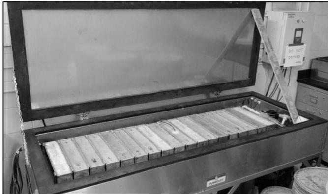
**Figure 5.17 Setup for Freezing and Thawing Concrete.**
