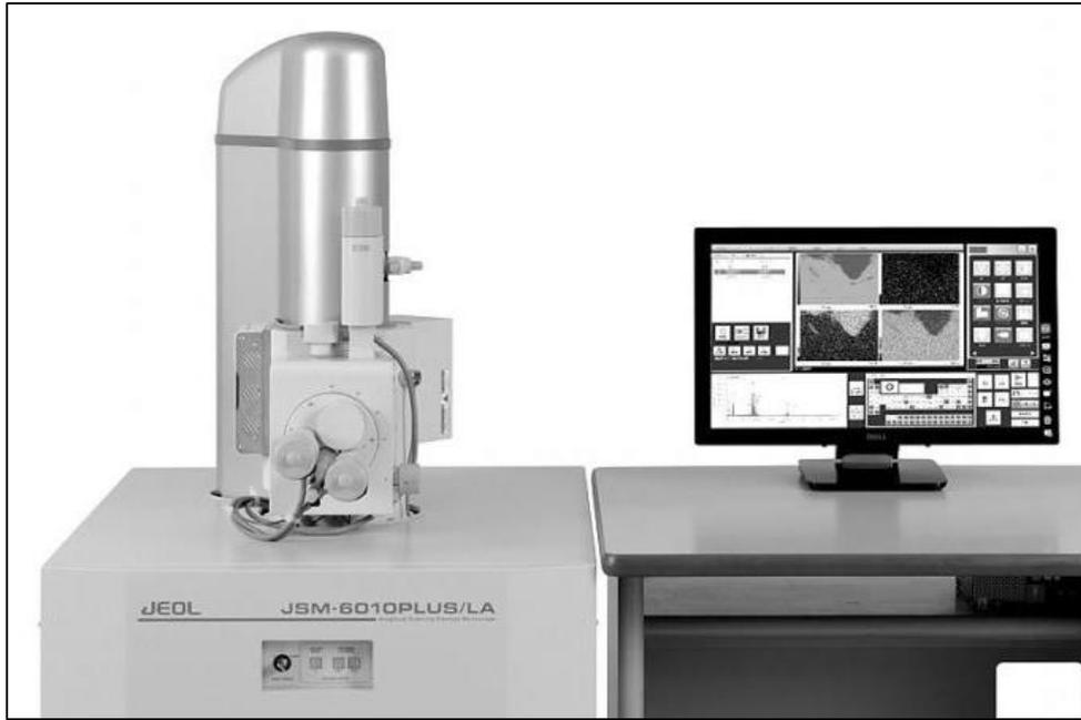
**Figure 5.4 JEOL JSM-6010Plus/LA Analytical Scanning Electron Microscope.**
