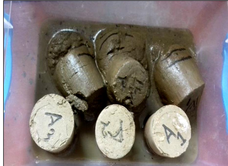
Figure 10. Comparison between treated and untreated soil based on water storage test. After 3 days, treated soil sample remains same as before with the increasing amount of weight and moisture content. That means, it just changed the soil structure internally and made it stronger. That's how, treated soil structure could survive even if there is water. The treated soil was not washed away like the untreated soil. It can be assumed that the absorbed water for treated sample may be chemically combined with the particle of clay surface and cannot swell because of alphasoil particle, that's why weight increases but no damage in each treated soil sample.
