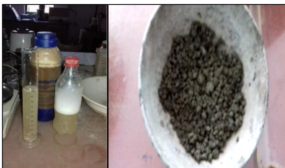
Figure 3. Treated soil sample by using alphasoil dilution. A ball was formed by hand with the material and dropped from 1m to the floor. As there were no cracks and fissures in this ball shaped sample, it was determined that the ball shaped sample was hardly formed, and the water content and material composition were in order. After stabilizing soil by alphasoil, different types of experiments such as standard proctor compaction test, unconfined compressive strength test, liquid limit and plastic limit test and water storage test were conducted to determine the performance of treated samples in comparison with untreated samples.
