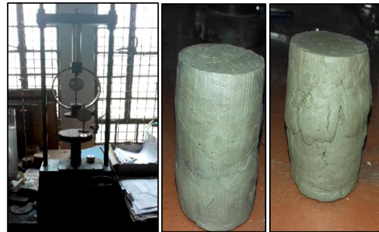
Figure 4. Compression testing machine. Treated soil sample before UCS testing and after testing. Treated soil sample was molded into a cylinder-shaped mold (2" diameter and 5" height). Deformation dial reading – 0.01mm, Load dial division – 0.00147 kN/div. Deformation dial gauge reading was recorded after every 60s.
