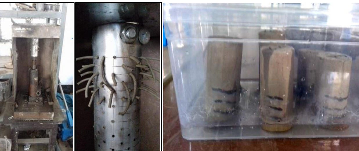
Figure 6. California Bearing ration testing machine. The mold with treated soil sample was pressed by load until no more water escaped out from the drainage holes. By opening the press-core, it was pumped out from the mold and dried in an oven for 3 hours at 70°C. Samples were provided with 3 marks (1cm-2cm-3cm) and weight of each sample was taken. It was filled with water in a water bath up to 1st mark.
