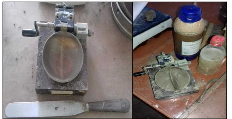
Figure 5. Grooving tool with spatula for LL and PL test. This test was performed for treated and untreated soil sample. For 25 blows, water content value was recorded and considered as liquid limit of the soil sample. This test was performed to know the plasticity index (PI) of treated and untreated soil.
