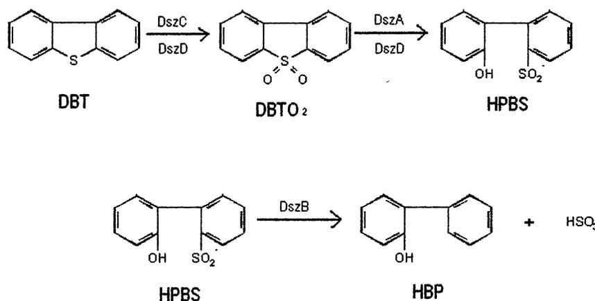
Figure 2. The dsz pathway for sulfur-specific desulfination of DBT.
