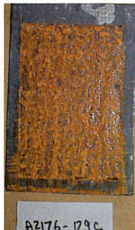
The inability of the lubricant to provide corrosion protection suggested formula changes were required. Efforts were made to retain the urethane resin and molysulfide combination due to the endurance life provided. Commercially available corrosion control additives, listed in Table 3.7, were incorporated into the formulation but did not improve the performance.
