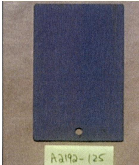
Unfortunately, the endurance life dropped from 90 minutes to seven with the addition of the acrylic. It was suspected that the acrylic may not bond effectively to molysulfide, causing reduced endurance life.
