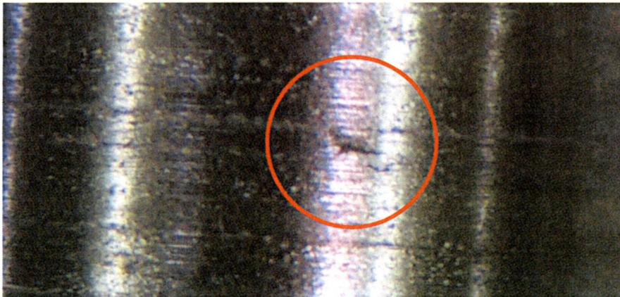
Optical microscopy revealed the burnished lubricant on Specimen 3 had a surface morphology that, upon closer inspection, was not homogenous. Figure 5.3 is a photograph of Specimen 3. The top section of the pin, after 30-minutes of extremem pressure wear, had a defined, macroscopic topography while the lower section appeared smooth and continuous.
