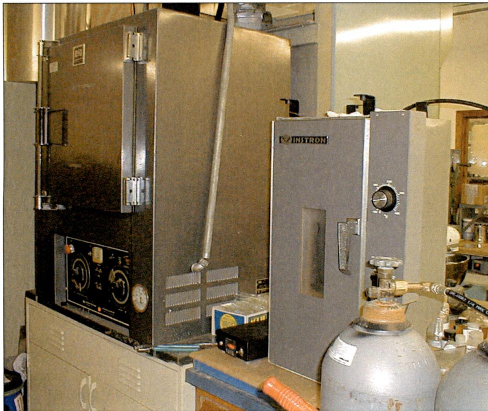
**Figure 3.16 Laboratory arrangement for thermal shock treatment: The left chamber is set at 260 °C and the right at negative 55 °C.**
