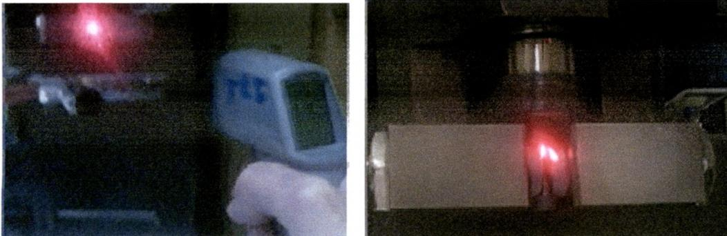
Torque on the Falex machine motor was simultaneously recorded to monitor lubricant performance. The pin surface temperature and machine torque were plotted as functions of time during the test. A plot in Figure 3.3 shows that under extreme pressure, temperature remains relatively constant between 105 and 140 °F during the required 60-minute duration. The temperature remained at least 200 °F below the decomposition point of the urethane resin.
