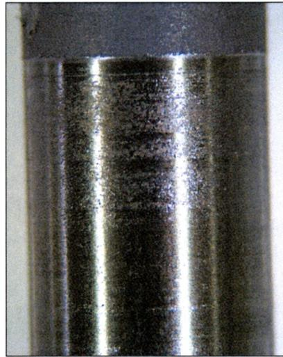
Specimen 4 was worn under extreme pressure conditions until lubricant failure. The photograph in Figure 5.4 shows distinct wear scars on the upper and lower sections. The lower scar on the specimen was deeper and more pronounced than the one above. The deep scar was the point of lubricant failure that caused an abrupt torque increase detected by the Falex machine.
