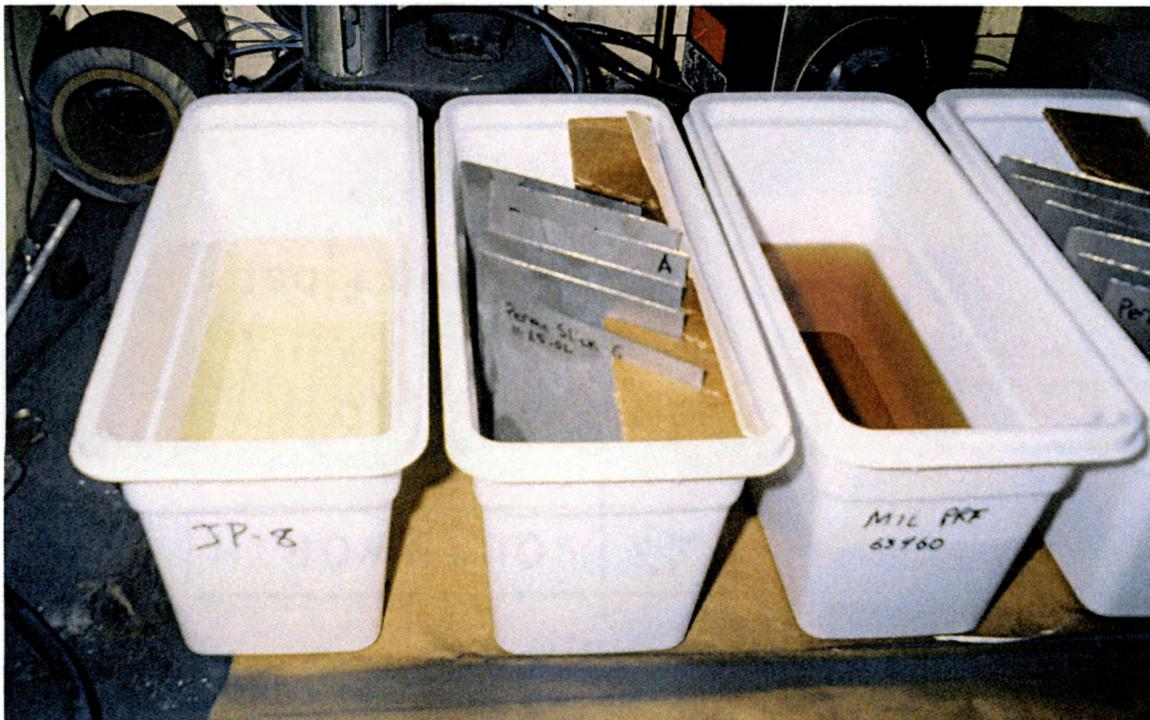
Panels coated with formulation A2200-91 were examined for fluid resistance and passed the requirements. Figures 3.12 and 3.13 are photographs of panels after immersion in the two most aggressive fluids, followed by required adhesion testing. Panels immersed in
