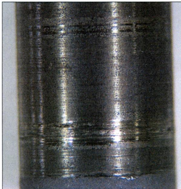
Optical microscopy was able to detect macroscopic defects on the coating surface that formed during the lubricant break-in period. It also showed the surface morphology of the burnished coating of Specimen 3. Finally, deep wear scars at the point of lubricant failure on Specimen 4 were closely inspected using microscopic analysis.
