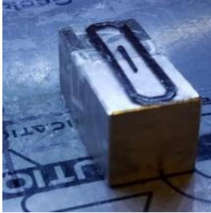
*Figure 3.2 MFAAM sample printed on NdFeB permanent magnets on top of 3-D printer's platform.*
