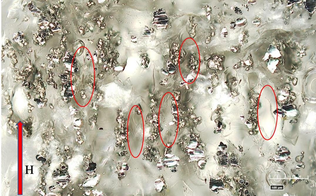
Figure 3.24 Cross sectional microscope image of the 5kOe transverse field 3-D printed filament. Chaining in the applied field direction is defined by the circled aggregates.
