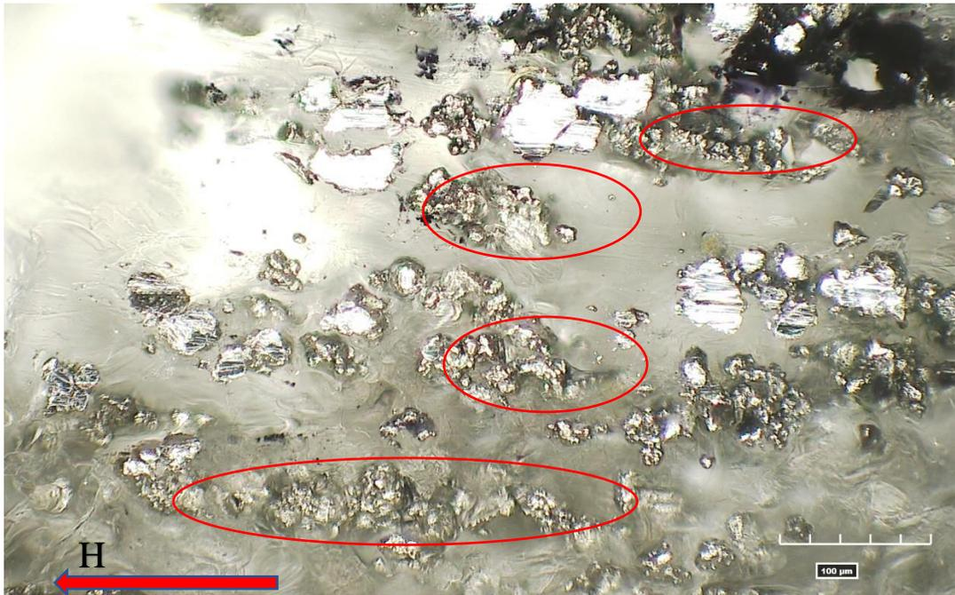
Figure 3.25 Cross sectional microscope image of the 8kOe parallel field 3-D printed filament. Chaining in the applied field direction is defined by the circled aggregates.
