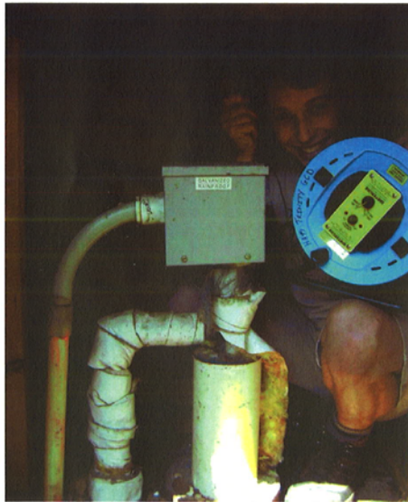
Figure 7. Water-Level Monitoring using an e-line
