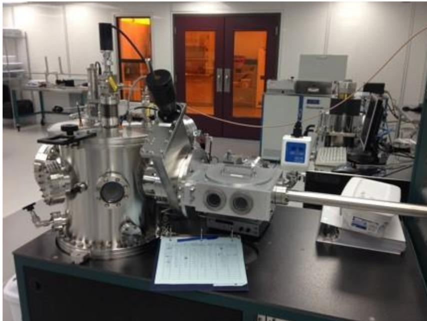
**Figure 6.1 AJA Sputtering System in the Cleanroom at Texas State University.**
