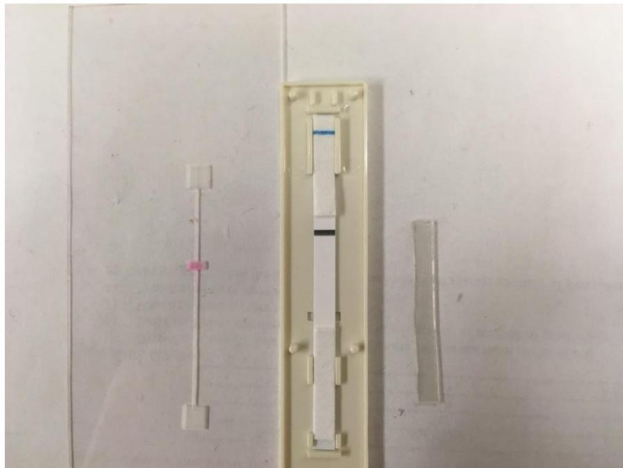
Fig. 44. Left: Compact PMMA device, Middle: Nitrocellulose device, Right: PMMA device the possible replacement of Nitrocellulose membrane only.
