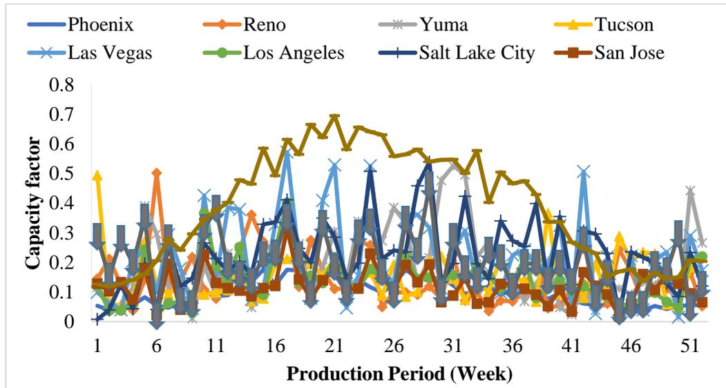
Figure 3.4: Weekly WT capacity factor for ten testing U.S. cities
