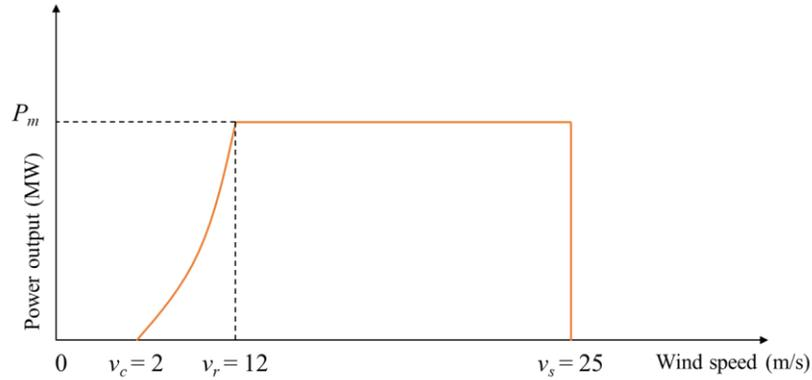
Figure 1.1: Wind turbine power curve
