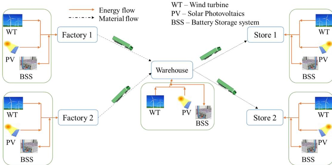
Figure 3.1: A Three-tier supply chain network with island microgrid systems
