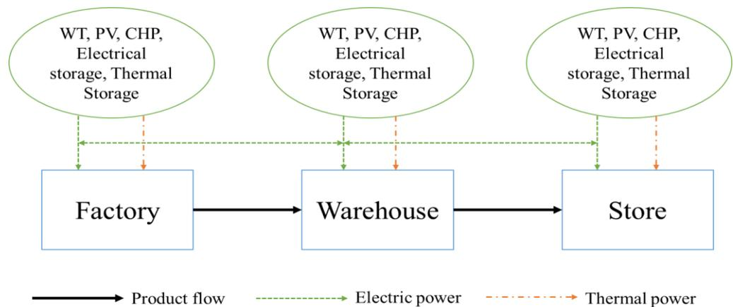
Figure 5.1: Electric and thermal power flow across different facilities
