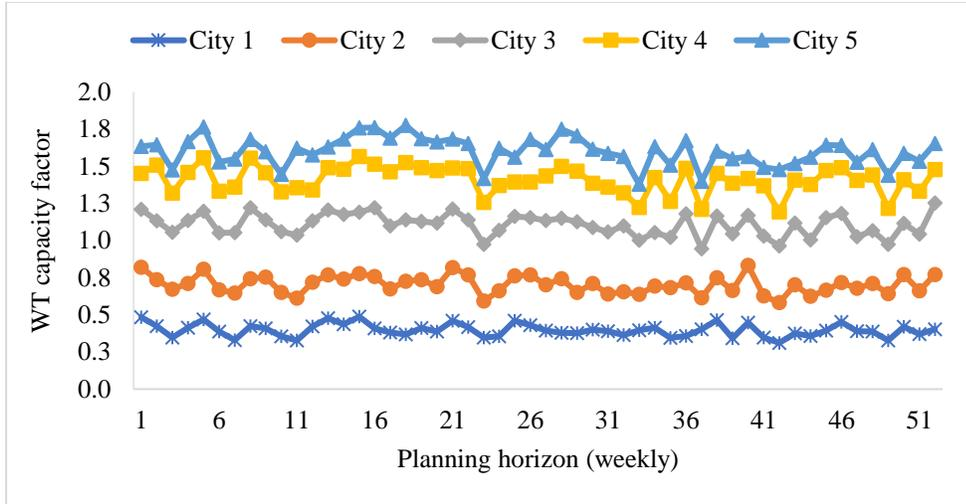
Figure 2.2: Wind turbine capacity factor for weekly planning
