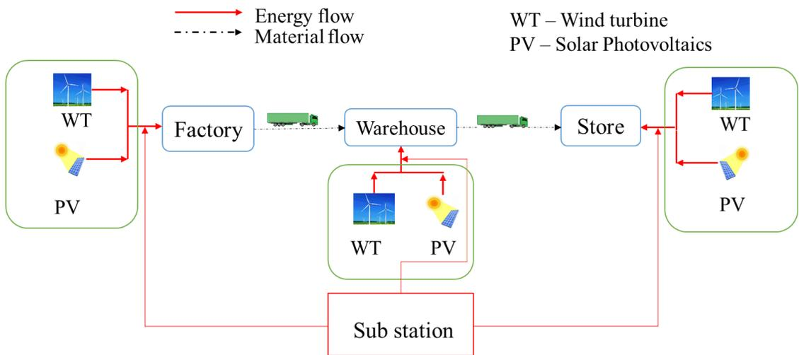
Figure 4.1: Multi-tier supply chain layout with grid connected microgrid
