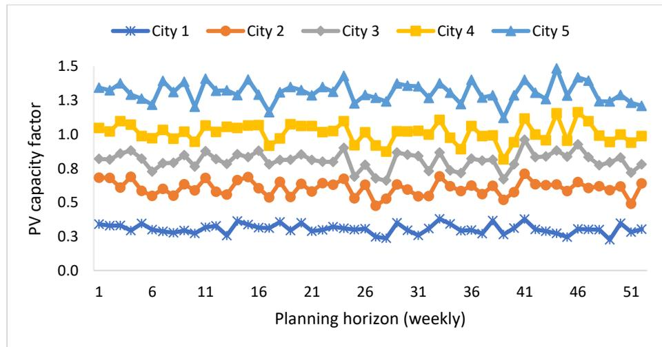
Figure 2.3: Solar PV capacity factor for weekly planning
