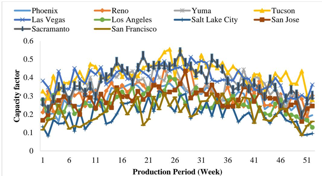
Figure 3.5: Weekly PV capacity factor for ten testing U.S. cities
