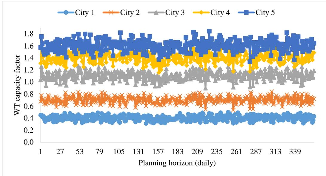
Figure 2.6: Wind turbine capacity factor for daily planning
