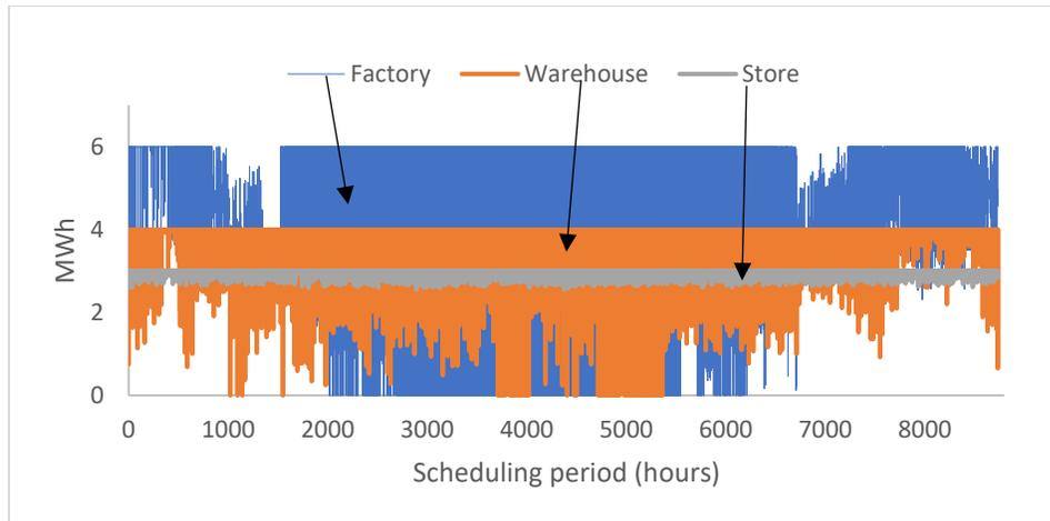
Figure 5.3: CHP electrical output for Case 1
