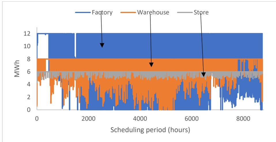
Figure 5.13: CHP thermal output for Case 5
