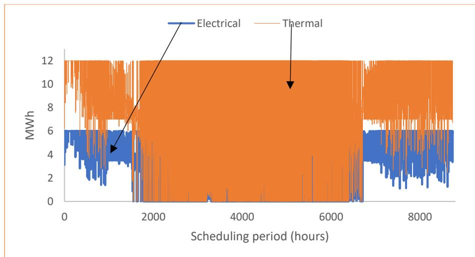
Figure 5.11: CHP outputs in Factory for Case 4
