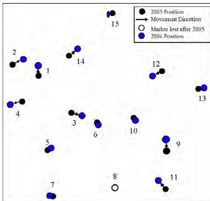
**Figure 63. Diagram of penny movement at Site I (Rachel), SP.**
