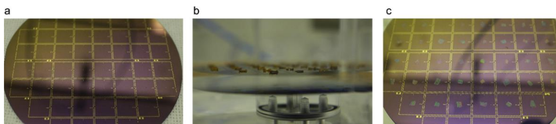
Figure 2.11. Photographs of wafer before the transfer (a), mediator film during the transfer (b), final product after the transfer (c). Retrieved from Kireev et al., 2016.
