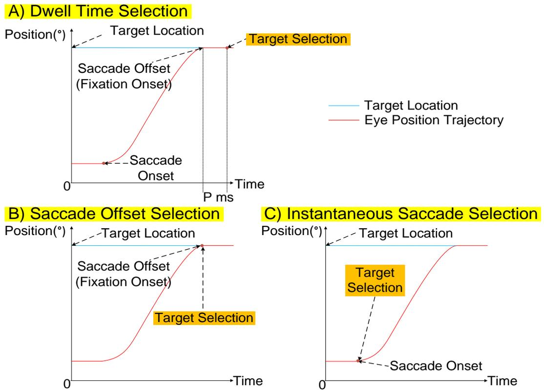
**Figure 1. Eye Movement Based Target Selections.** a) Dwell Time b) Saccade Offset c) Instantaneous Saccade.
