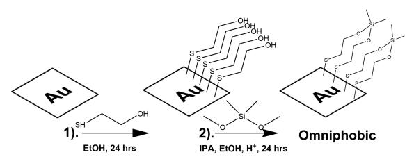
Figure 17. 1) Synthesis of the 2-mercapto ethanol-thiol coating, and 2) Formation of the omniphobic surface.
