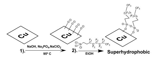
Figure 6. Synthesis of the superhydrophobic coating
